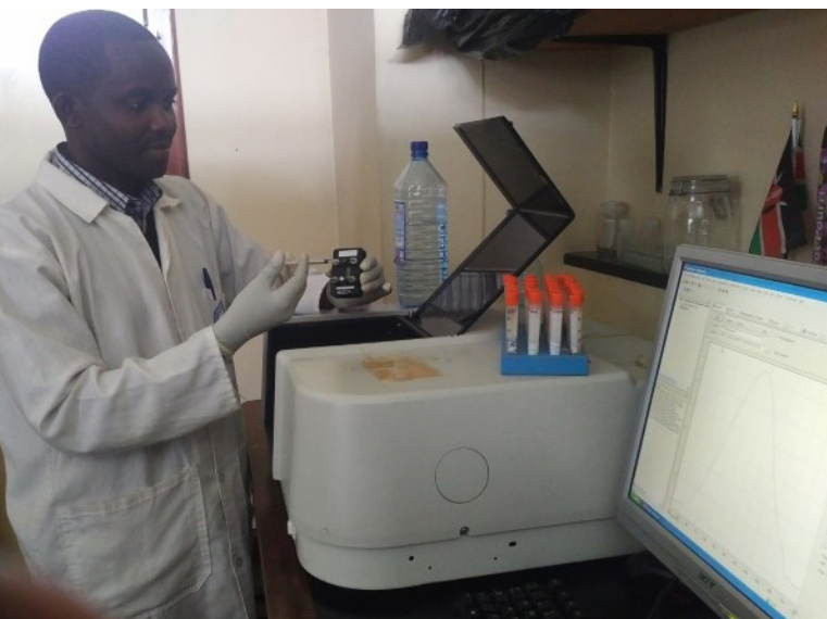
A technician analysing deuterium samples at a Fourier transform infrared spectrometer laboratory in Kenya. (Photo: C. Mwangi and S. Oiyee)
