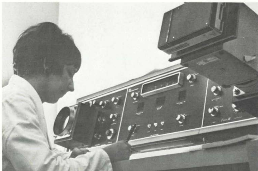
The control desk for a scintillation camera for viewing concentration of radioactivity – WHO
