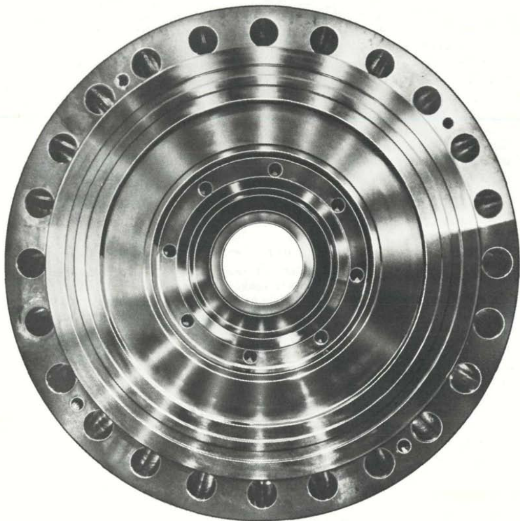
Stainless steel sculpture — the main flange for a Westinghouse nuclear coolant pump gleams like a piece of industrial pop art as it undergoes inspection. The flange, weighing 14,500 pounds, was carved from a single piece of stainless steel and machined to tolerances as low as two-thousandths of an inch . . . Westinghouse
