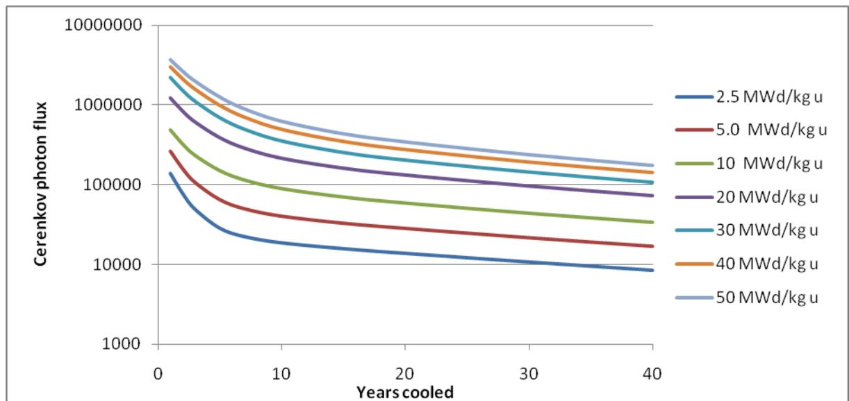
Fig. 8. Theoretical photon flux (intensity) for fuels of differing burnup and cooling time
