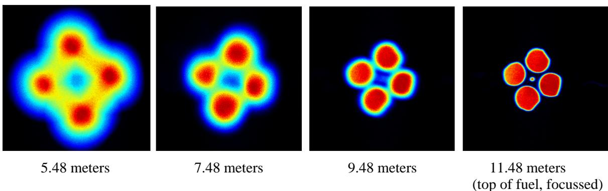
*Fig. 3. UV light images of CLS as a function of distance from DCVD in a fuel bay*
