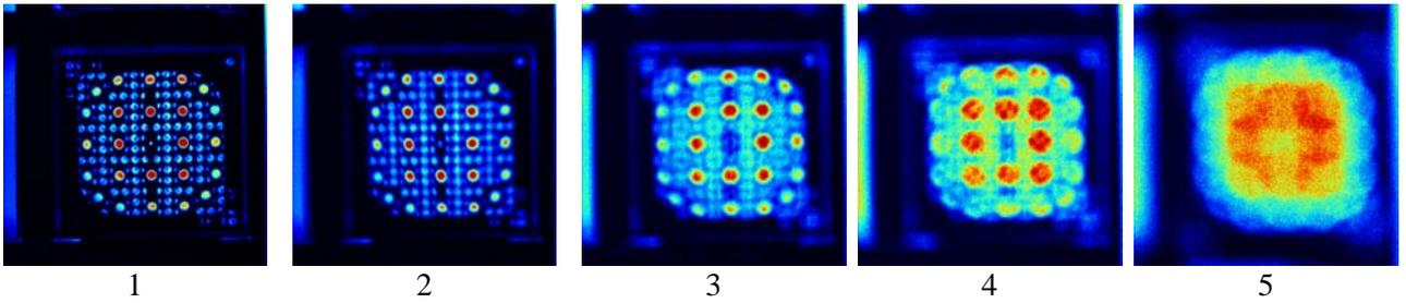
Fig. 5: Progressively defocused images of a PWR fuel
