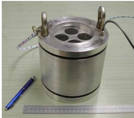
*Fig. 1. Calibration light source*
