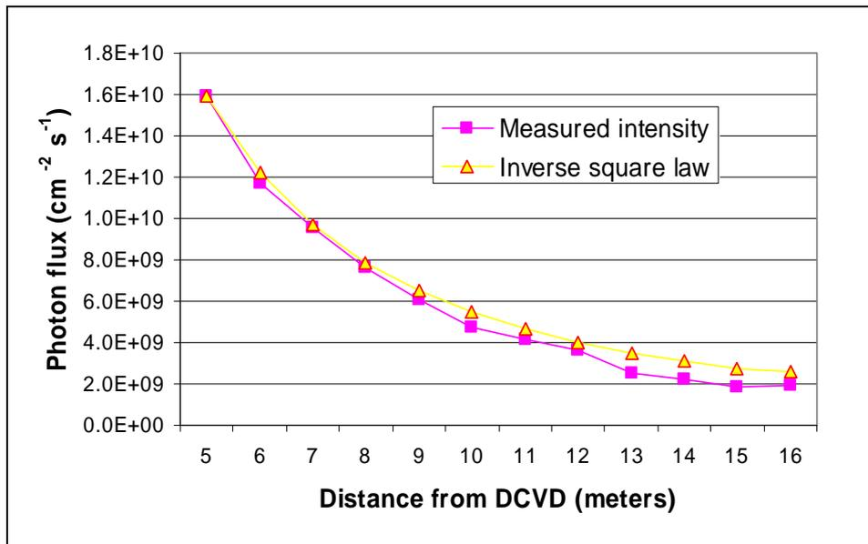
Fig. 4: Calibration light source intensity as a function of distance from DCVD
