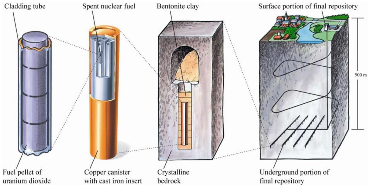
FIG. 16. The Swedish concept for the disposal of spent nuclear fuel as an illustration of the multi-barrier concept.
