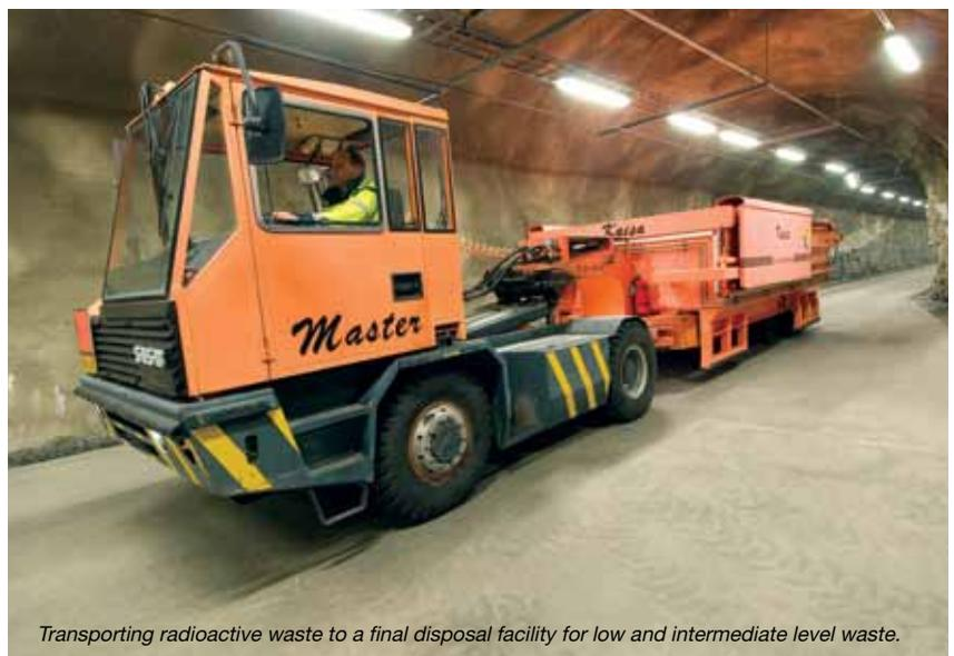
*Transporting radioactive waste to a final disposal facility for low and intermediate level waste.*
