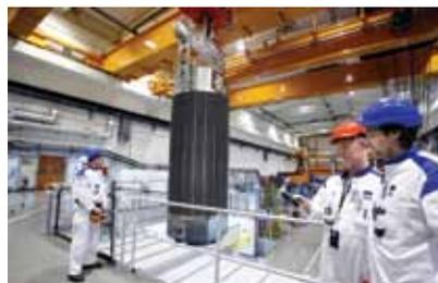
*After removal from the reactor, the fuel is highly radioactive. After a few years of cooling, the spent fuel can be transported to the interim storage facility.*
