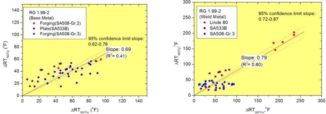
Fig. 2. Transition temperature shift data from surveillance tests compared with RG-1.99 Rev.2 model prediction
