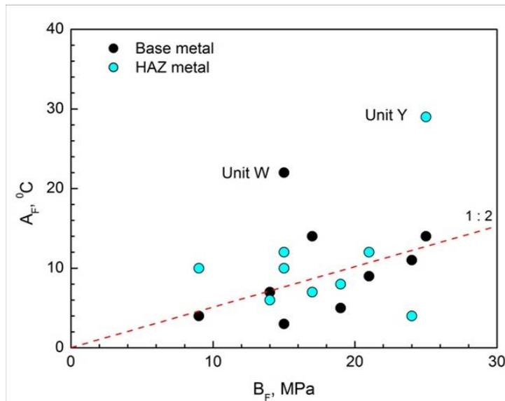
Fig. 4 Radiation hardening ( $B_F$ ) to embrittlement ( $A_F$ ) correlation for HAZ and base metal
