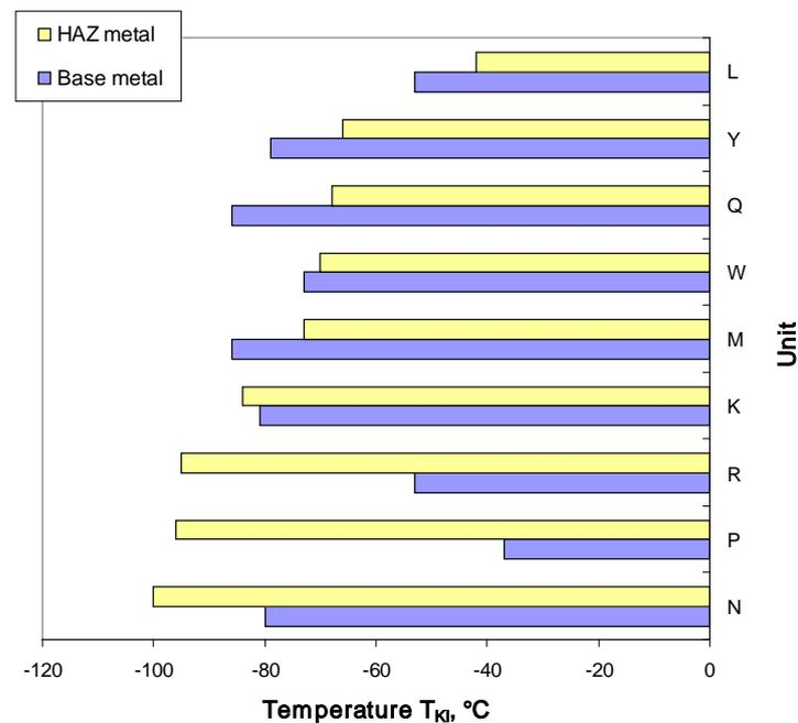
Fig. 2 Transition temperature  $T_{KI}$  for HAZ and base metal in unirradiated condition
