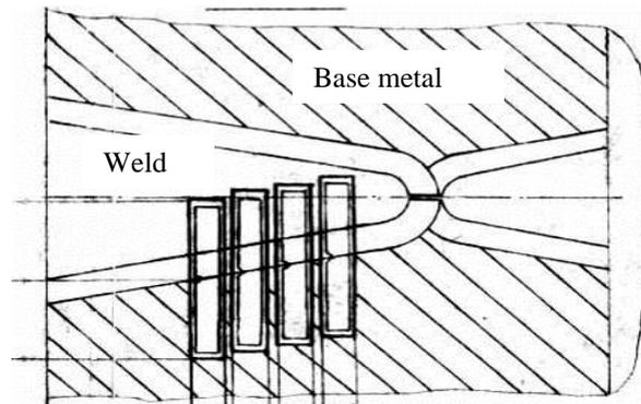
Fig. 1 Position of HAZ specimens relative to welds
