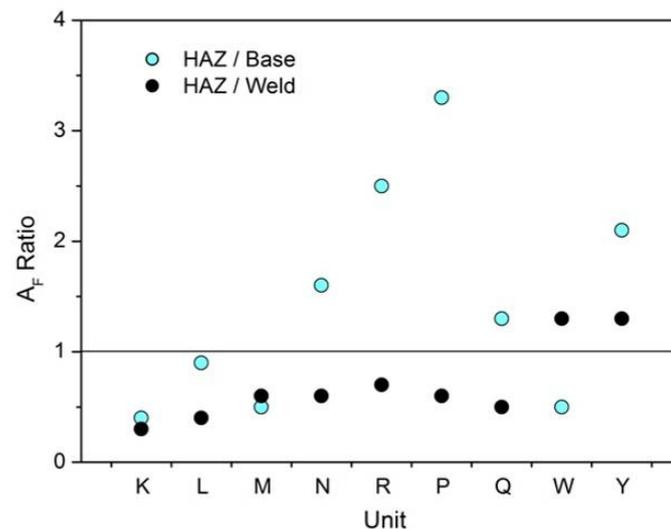
Fig. 3 Radiation embrittlement rate for HAZ relative to base and weld metal
