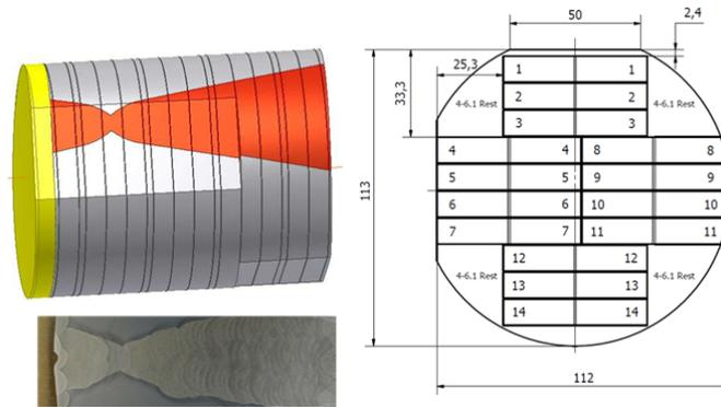
Fig. 1 Picture and cutting scheme of trepan 4-1.
