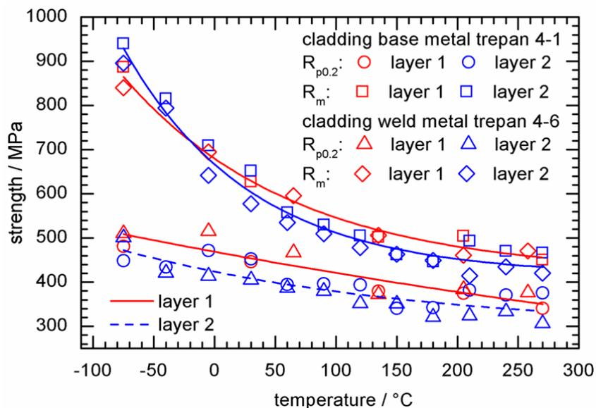
Fig. 3 Tensile strength characteristics of the cladding layers 1 and 2 vs. temperature.
