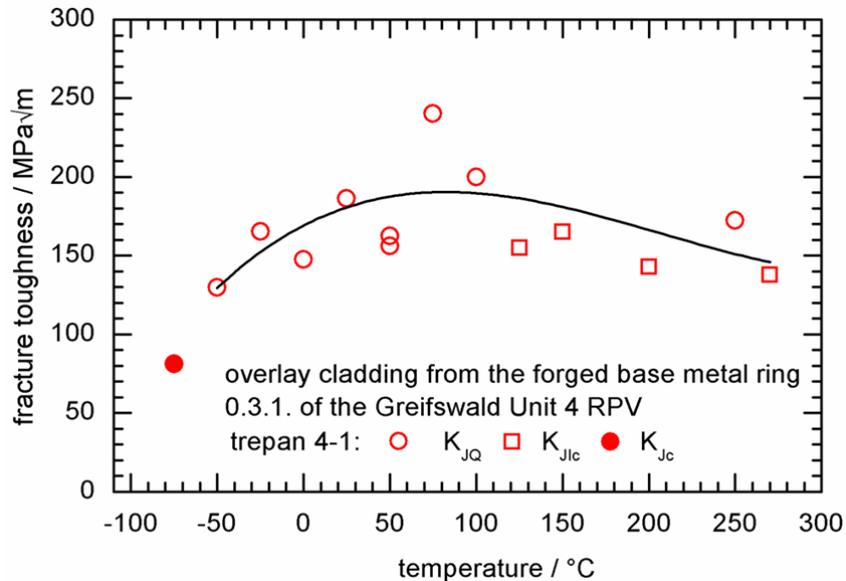
Fig. 6 Crack initiation fracture toughness values,  $K_{JQ}$ , vs. temperature of the investigated cladding from the forged base metal ring 0.3.1. of the Greifswald Unit 4 RPV.
