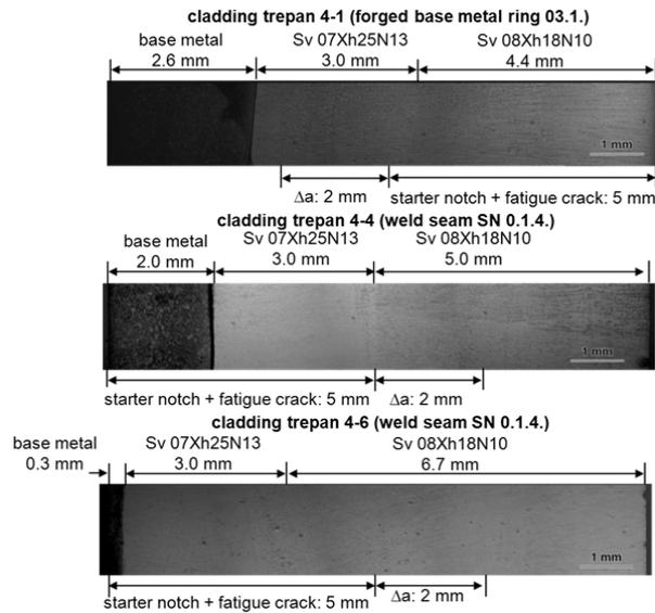
Fig. 4 Overview about the structure of the investigated overlay cladding from the individual trepans and the location of the crack tip.
