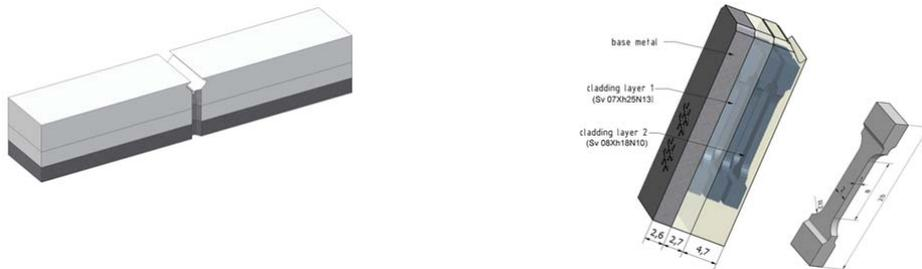
Fig. 2 Charpy size SE(B) specimen and scheme of the machining of sub-size tensile specimens from broken halves.
