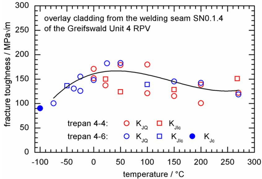
Fig. 5 Crack initiation fracture toughness values,  $K_{JQ}$ , vs. temperature of the investigated overlay cladding from the welding seam SN0.1.4. of the Greifswald Unit 4 RPV.
