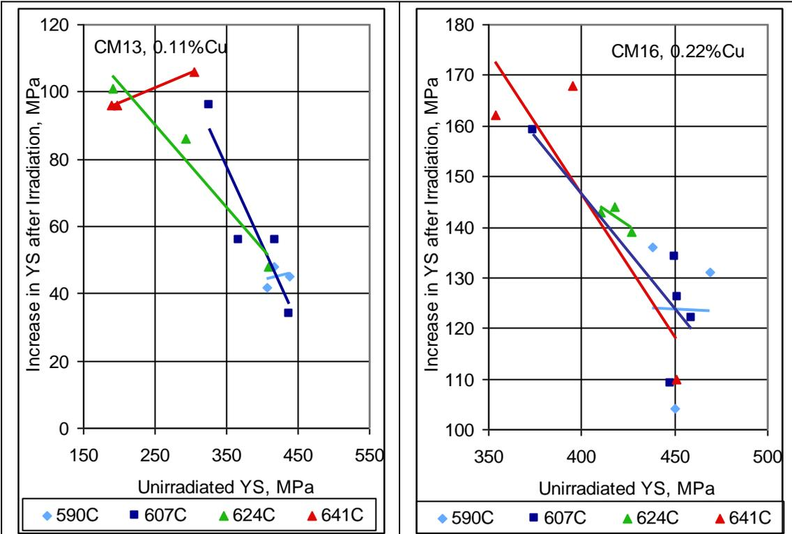
**Figure 4 The effects of stress relief temperature on the irradiation sensitivity of medium copper, medium nickel steels CM13 and CM16 related to unirradiated strength**
