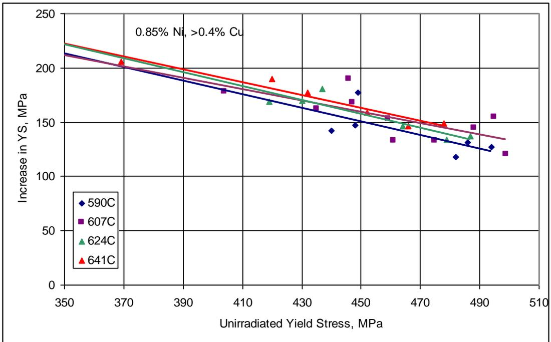
**Figure 3 The effect of unirradiated strength on the irradiation sensitivity of high copper, medium nickel steels related to stress relief temperature**
