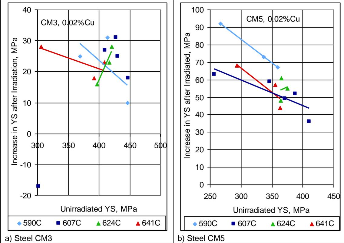
**Figure 5 The effects of stress relief temperature on the irradiation sensitivity of low copper, medium nickel steels CM3 and CM5 related to unirradiated strength**
