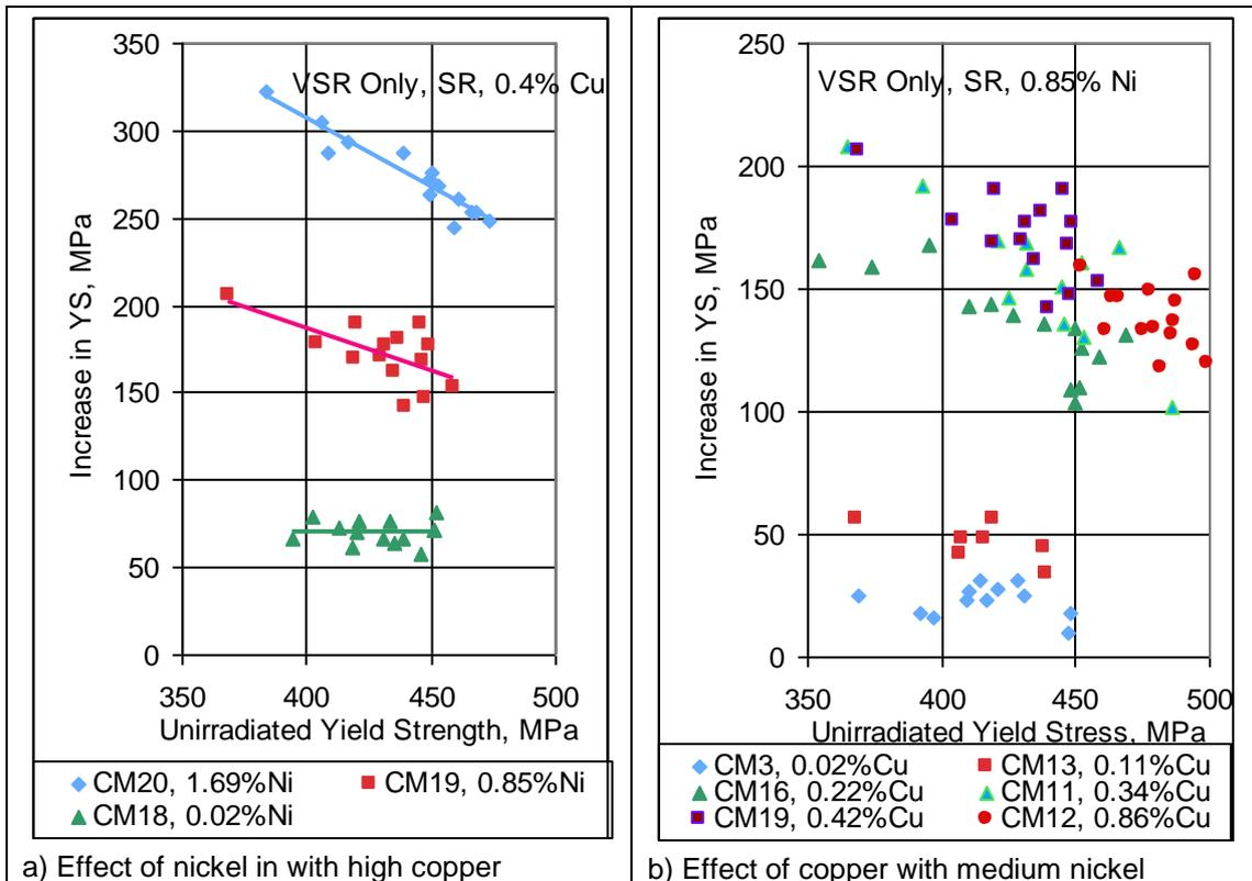
**Figure 1 Effect of unirradiated yield strength on irradiation induced yield strength increases**
