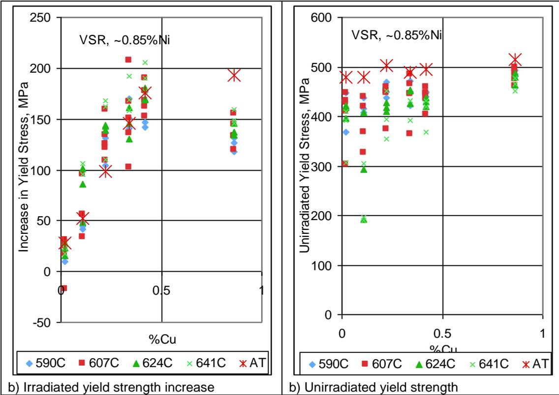
**Figure 2 Effect of copper on unirradiated yield strength and increase in yield strength after irradiation in medium nickel steels (AT = As Tempered)**
