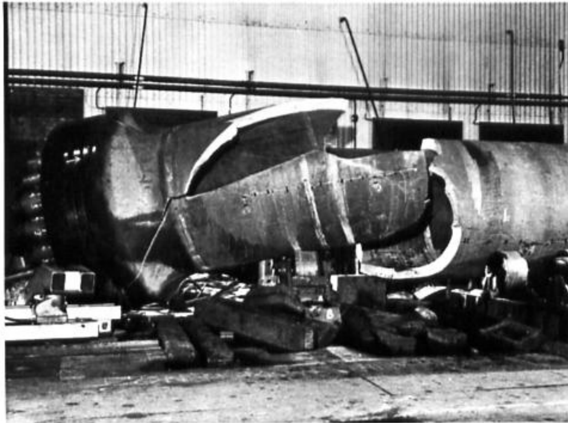
Fig. 1.12. Failure by brittle fracture of thick-walled cylindrical pressure vessel during hydraulic test (By courtesy of John Thompson Ltd., Wolverhampton)
