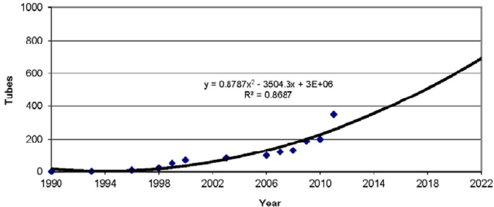
**Fig-1: Prediction (polynomial) of Total Plugged Tubes in Six SGs at KANUPP**
