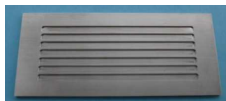
Straight channels on sodium side
