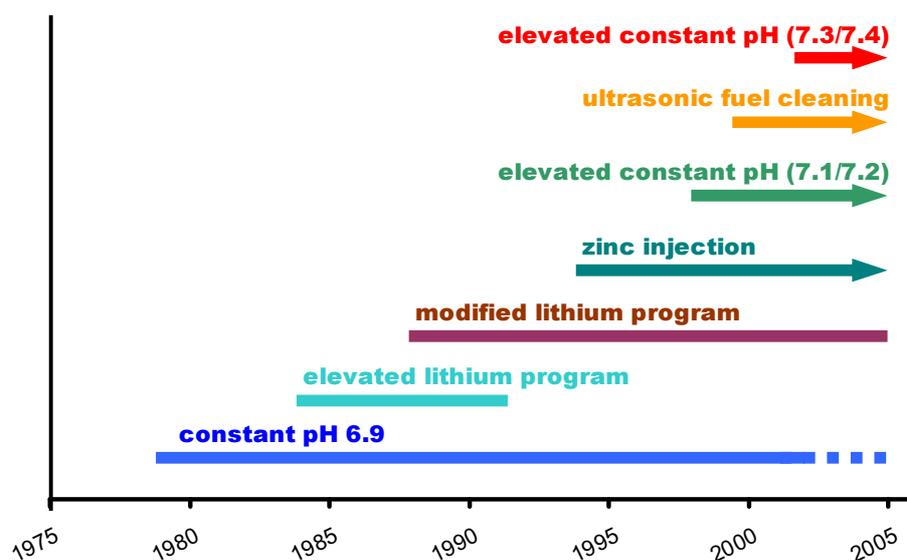
Figure 3. Evolution of recommended PWR water chemistry
