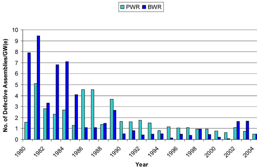
Figure 5. Fuel failure rates in US plants.
