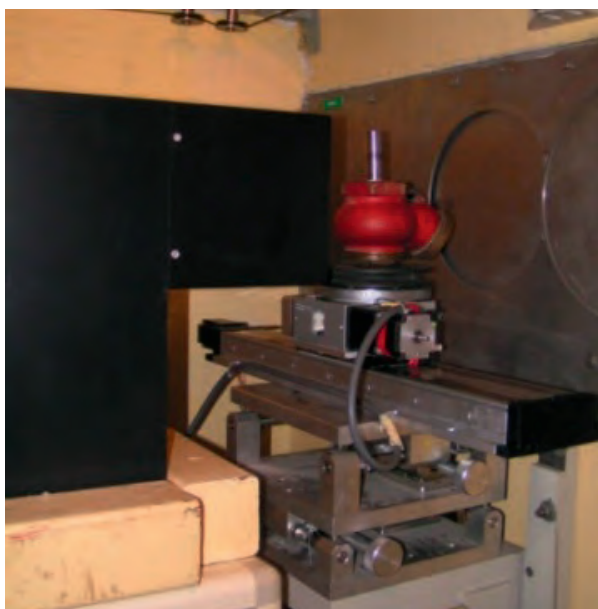
FIG. 2. A digital neutron imaging facility (left) licensed at the ETRR-2 reactor in Egypt. This state of the art installation will provide 2-D and 3-D non-destructive testing capabilities for various applications. On the right is a reconstructed image of a defective valve.
