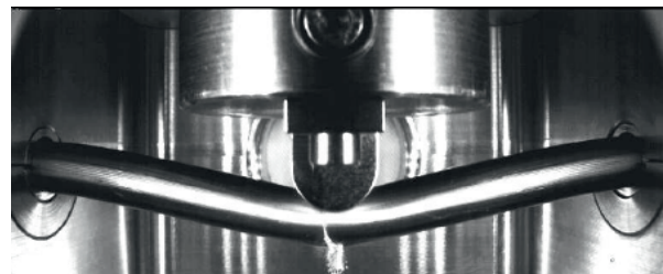
FIG. 3. High speed photograph showing impact testing of a fuel rod.
