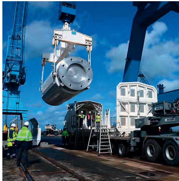
FIG. 3. A transport cask containing radioactive material being loaded for shipment.
