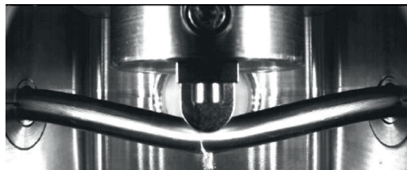
FIG. 3. High speed photograph showing impact testing of a fuel rod.
