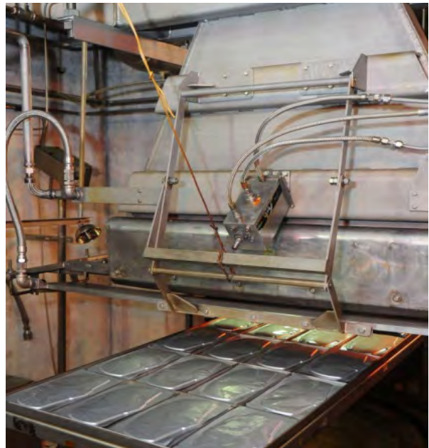
FIG. 3. Radiation processing (cross-linking and sterilization) of nanocomposite, bio-based hydrogels for biomedical applications at Nuclear Malaysia.
