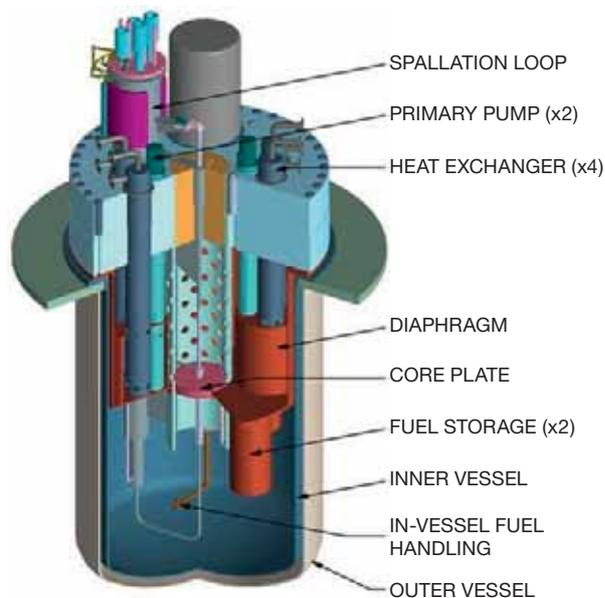
FIG. 3. Schematic drawing of the MYRRHA ADS.
