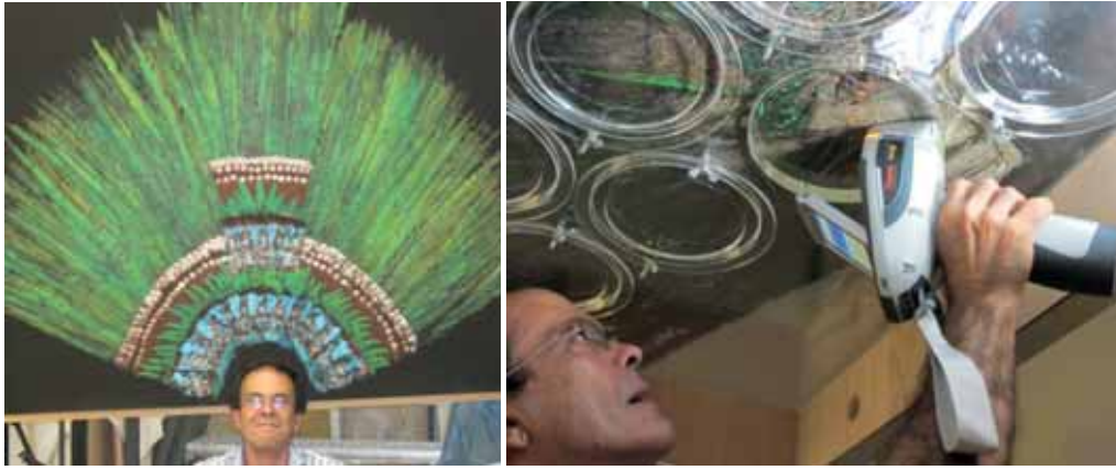
FIG. 5. A 16th century Mexican headdress (left) being examined with a hand-held X ray fluorescence spectrometer (right).
