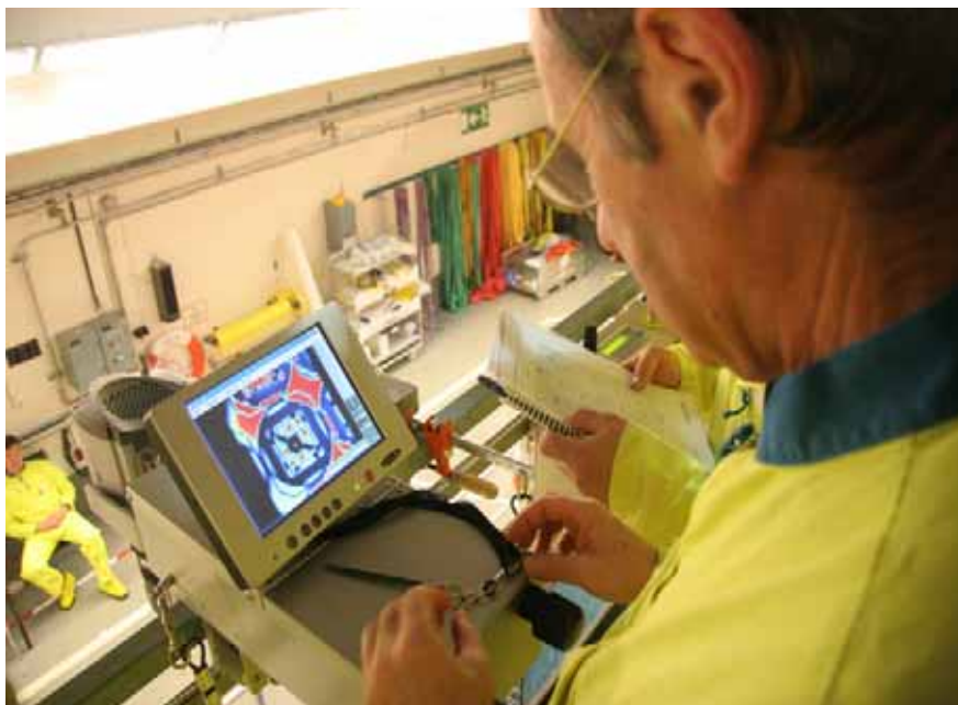
FIG. 2. Verification of spent fuel using a digital Cerenkov viewing device.
