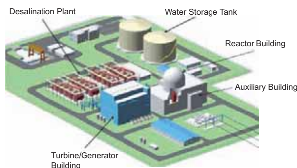
FIG. 2. An example of an SMR — the System Integrated Modular Advanced Reactor (SMART) in the Republic of Korea (photo credit: KAERI).
