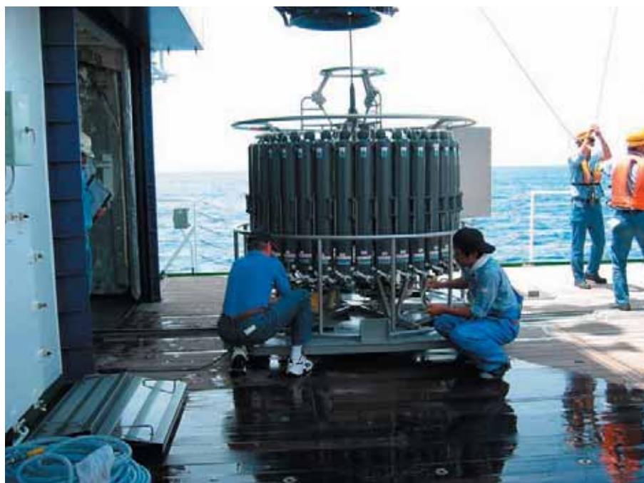
FIG. 2. Sampling of seawater and particles for the measurement of natural radiotracers.
