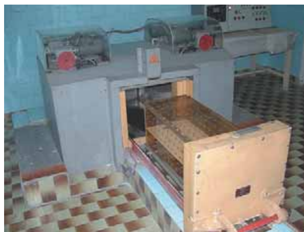
FIG. 1. An old irradiator with caesium-137 sources in Bulgaria before decommissioning.
