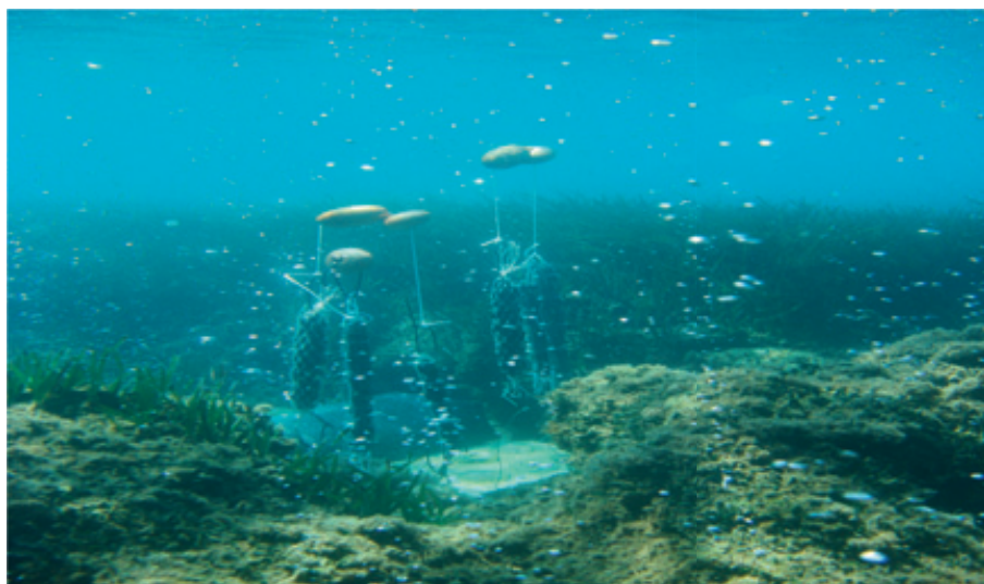
FIG. 1. Ocean acidification simulations included a transplantation experiment at volcanic carbon dioxide vents at Ischia Island in the Gulf of Naples using the commercially important mollusc Mytilus galloprovincialis .
