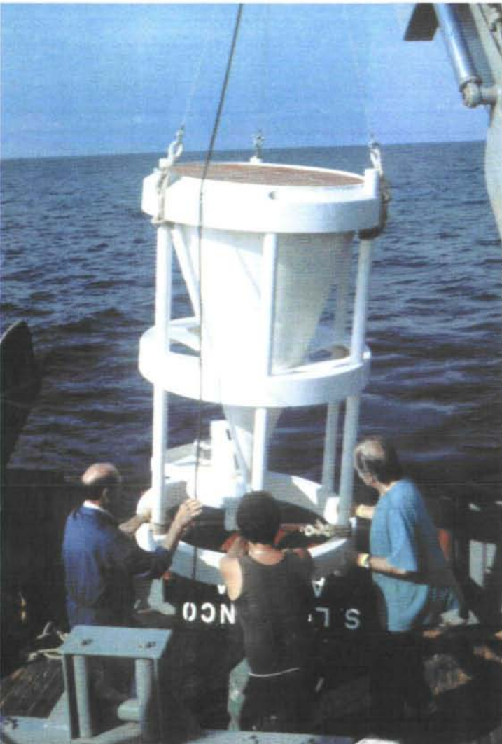
Top: As part of an IAEA-MEL training course in Istanbul in November 1994, scientists collect sediment samples in the Marmara Sea using the University of Istanbul's ship. Left: A team of IAEA-MEL scientists deploy a sediment trap such as the ones used during their post-Chernobyl marine studies. Above: Typical particles collected in sediment traps include oval, rectangular, and cylindrical fecal pellets produced by zooplankton that are actively feeding on micro-organisms. (Credits: IAEA-MEL).
