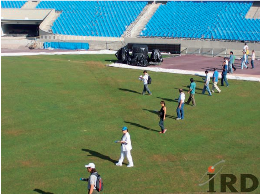
FIG. 10. Survey of the João Havelange soccer field using a line of RIDs and backpack.
