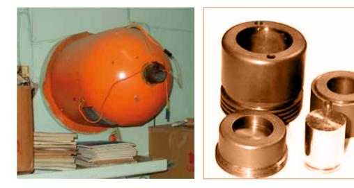
Developed in 2004, the **mobile hot cell** is a device which may be locally assembled and used to recover radioactive sources in States without proper facilities and in States where recovery would otherwise be very difficult. In the mobile hot cell, the sources are removed from their respective shielding and then moved into special capsules, specifically designed for safe and secure long term storage. *This process ensures that the sources will not fall into the wrong hands*.
