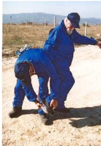
**Checking for contamination after finished work at Borovac**
