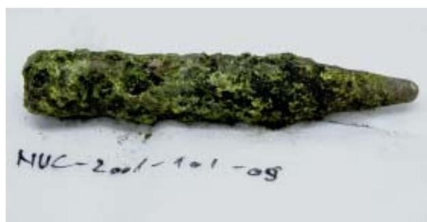
**Corroded penetrator collected at Pljackovica**
