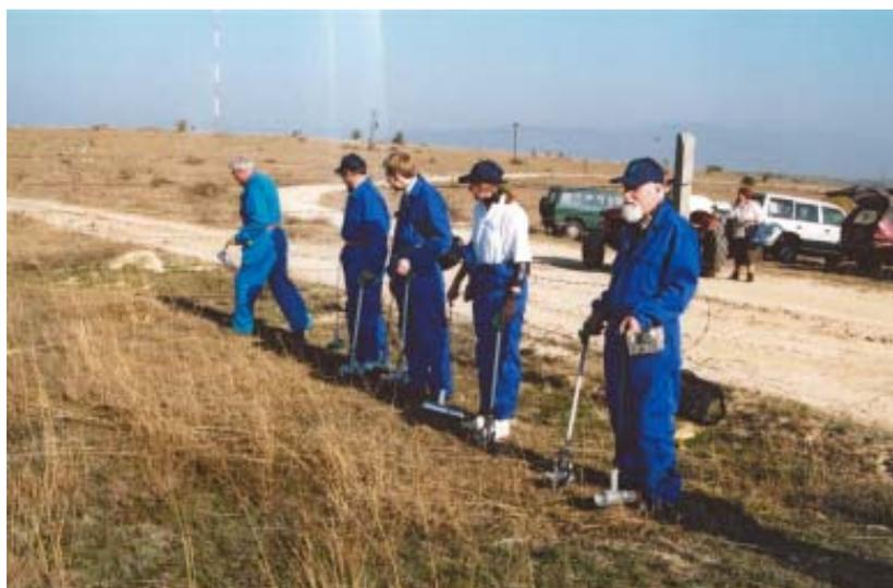
The surveys of radiation in the environment were made using beta and gamma instruments held close to the ground, with the team members often employing the ‘line-up’ survey technique described in Appendix C ‘Methodology and Quality Control’.
