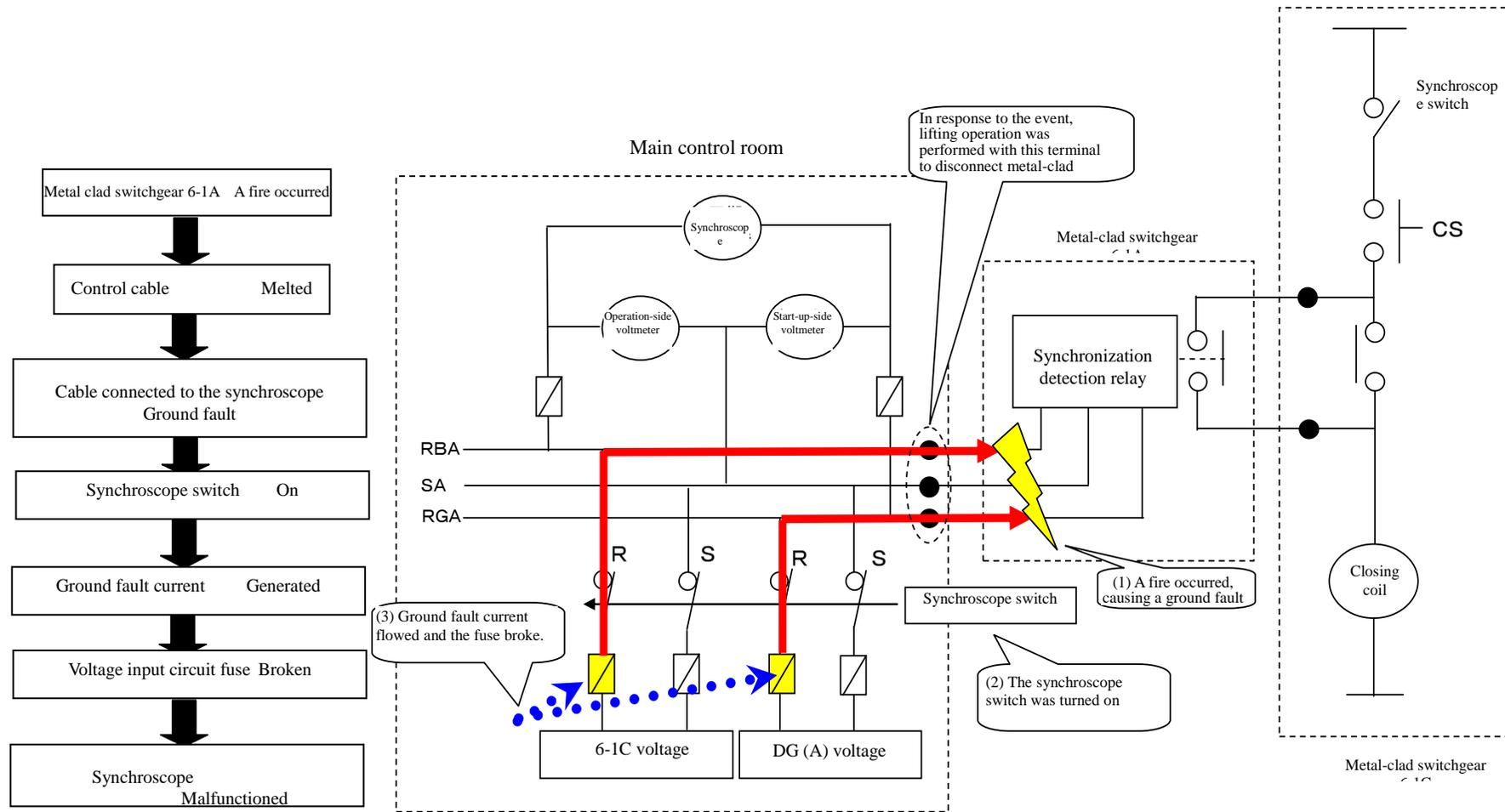
Fig. II-2-152 How the synchroscope malfunctioned
