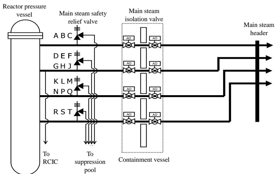
Figure II-2-93 System Diagram of Main Steam Safety Relief Valve (Units 2-4)
