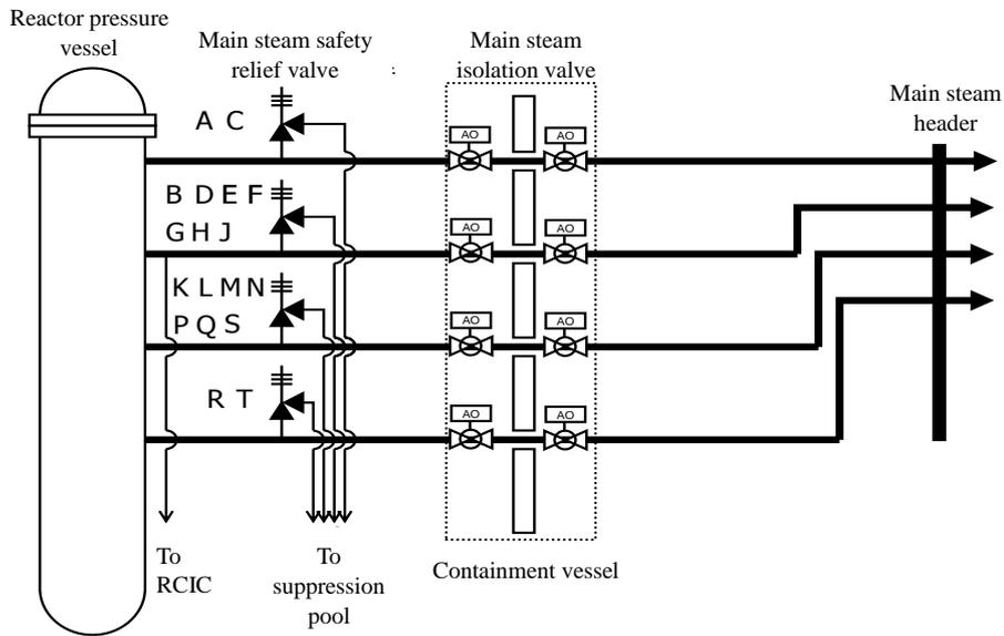
Figure II-2-92 System Diagram of Main Steam Safety Relief Valve (Unit 1)
