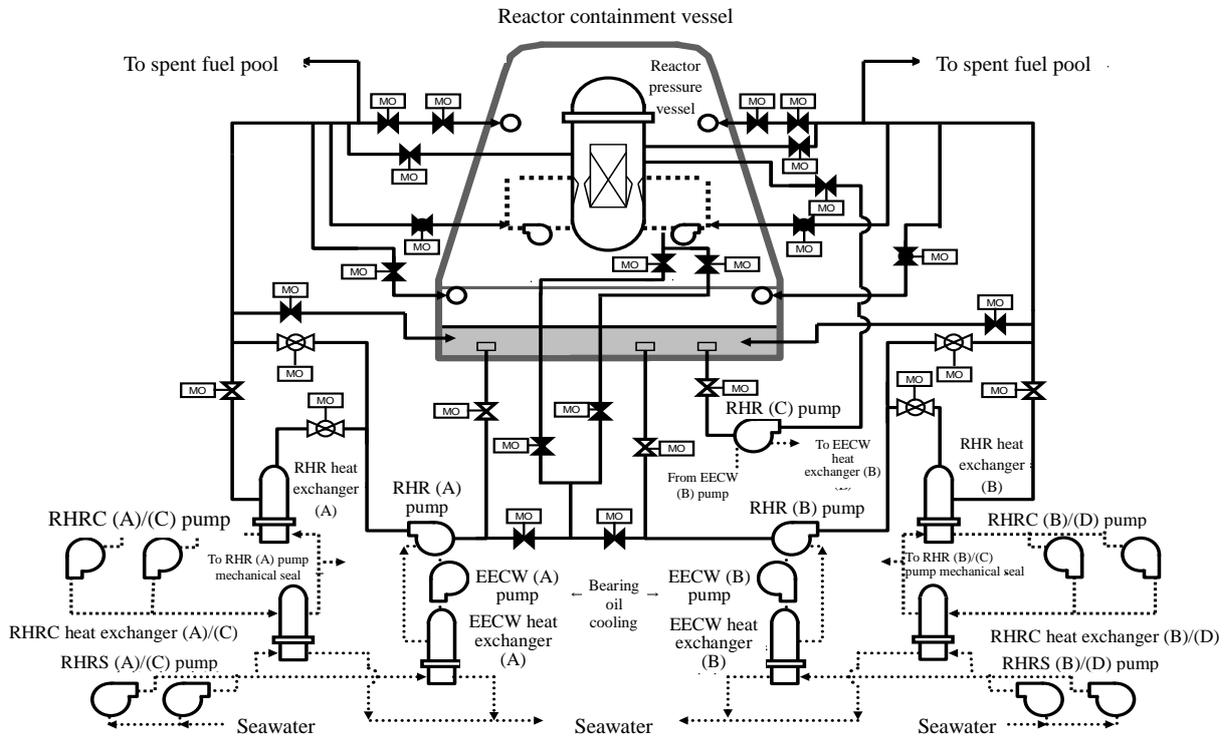
Figure II-2-95 System Diagram of Residual Heat Removal System (Unit 2)
