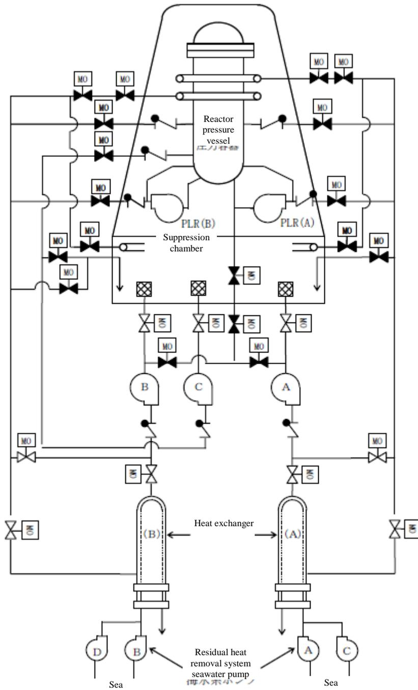
Figure II-2-157 System Configuration Diagram of Residual Heat Removal System
