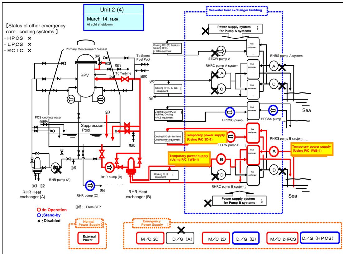
Figure II-2-113 Schematic Diagram of Station Status [2F-2] (Part 2)
