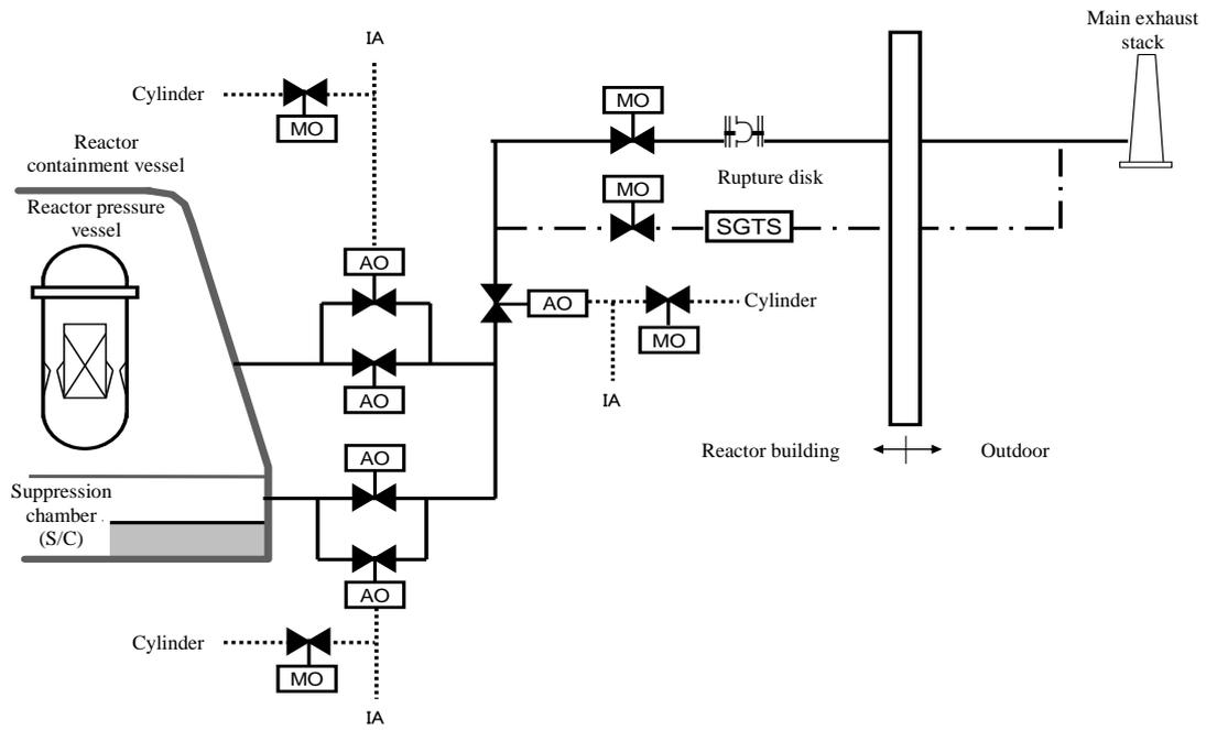
Figure II-2-105 System Diagram of PCV Vent (All Units)
