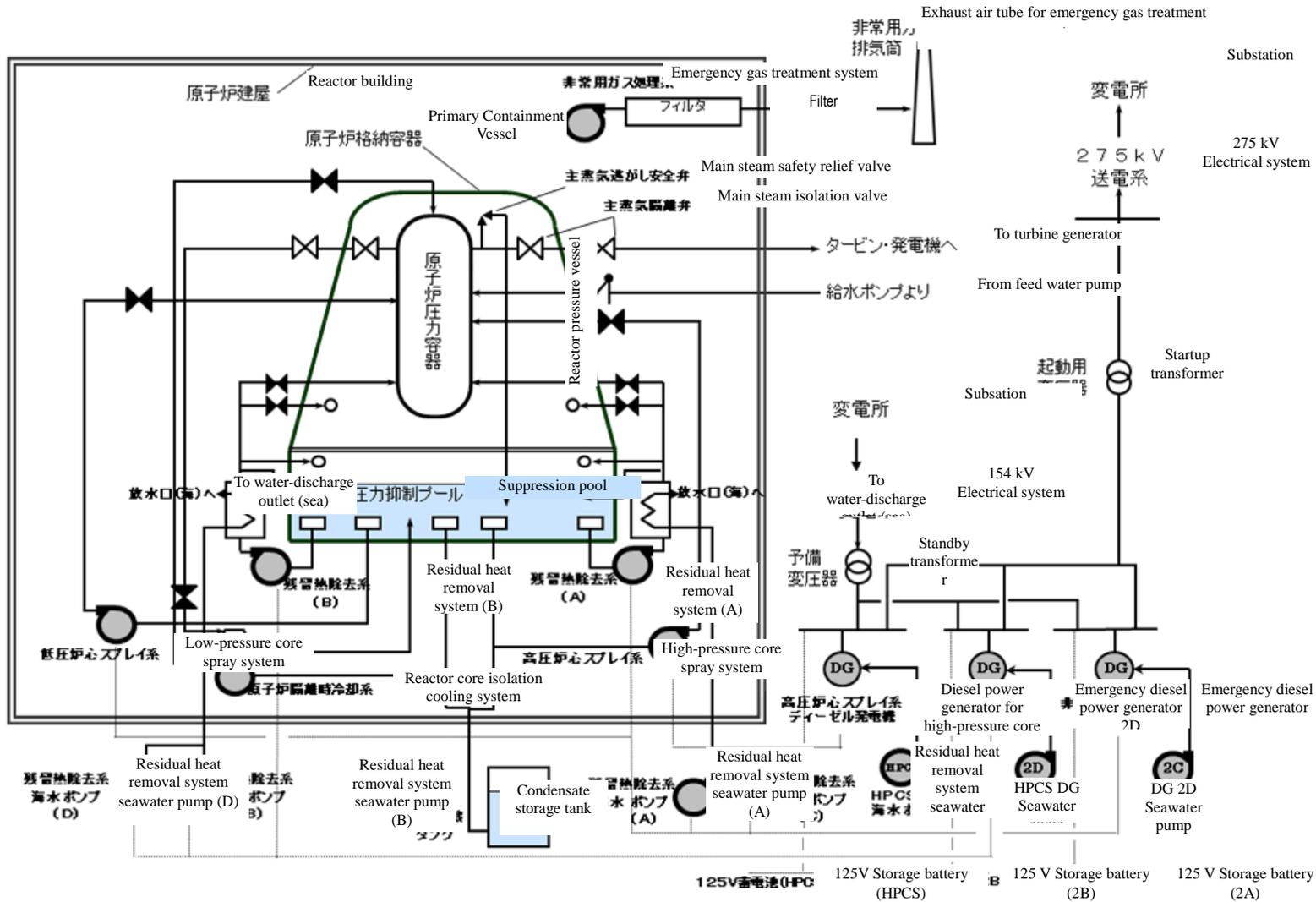
Figure II-2-156 System Configuration Diagram of Tokai Dai-ni NPS
