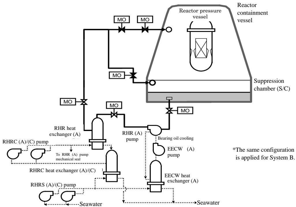
Figure II-2-101 System Diagram of PCV Spray (D/W and S/C)
