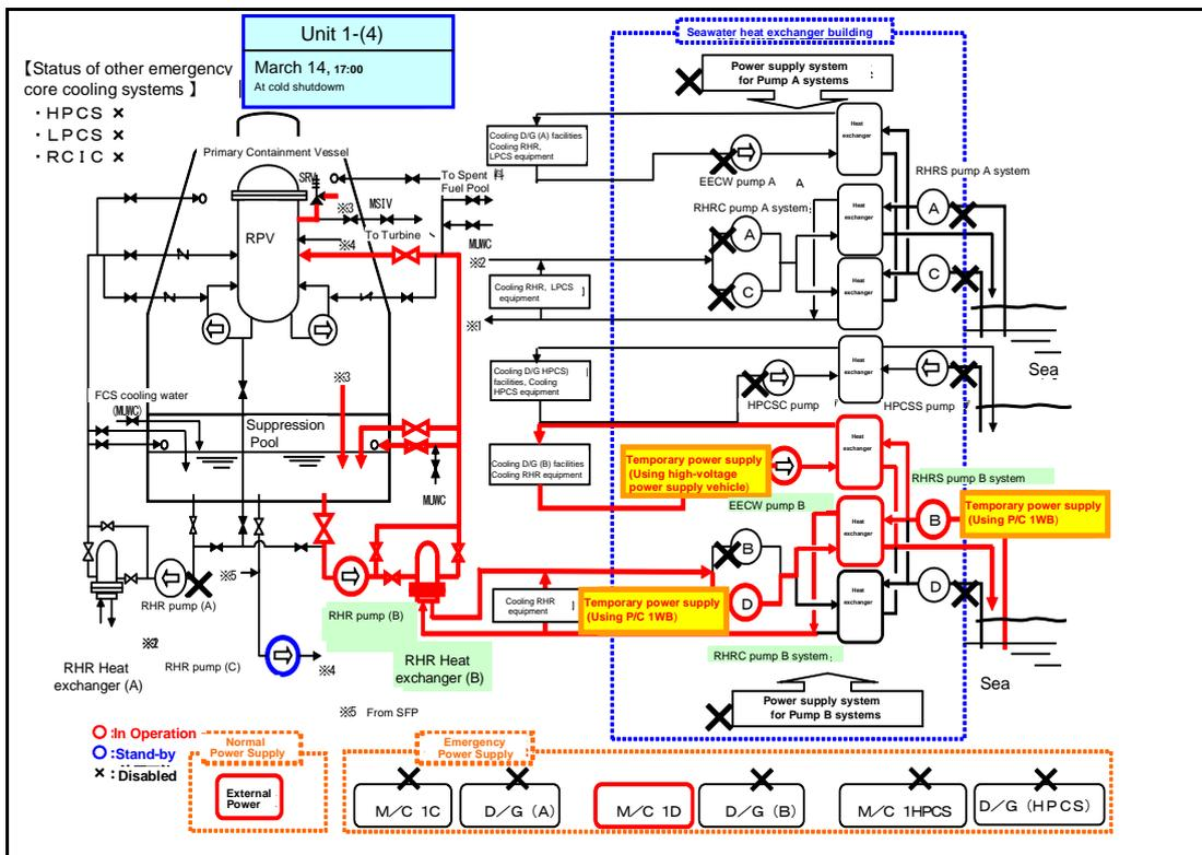
Figure II-2-108 Schematic Diagram of Station Status [2F-1] (Part 2)
