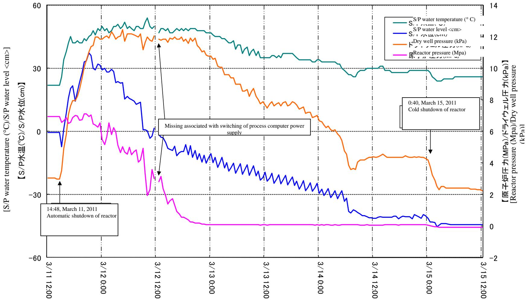
Figure II-2-163 Variation of Main Parameters (from March 11 till March 15) (No. 2)
