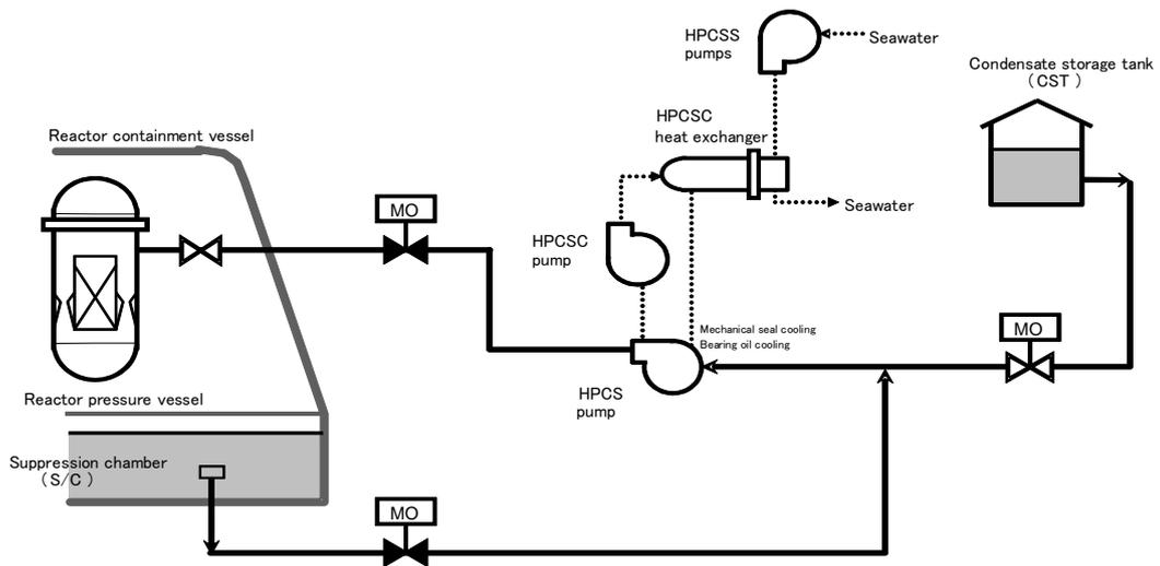
Figure II-2-88 System Diagram of High Pressure Core Spray System (Units 2 and 4)
