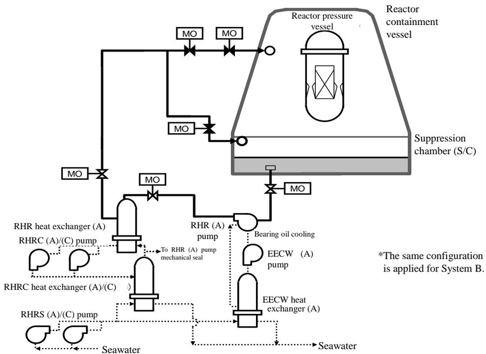
Figure II-2-102 System Diagram of PCV Spray (D/W and S/C)
