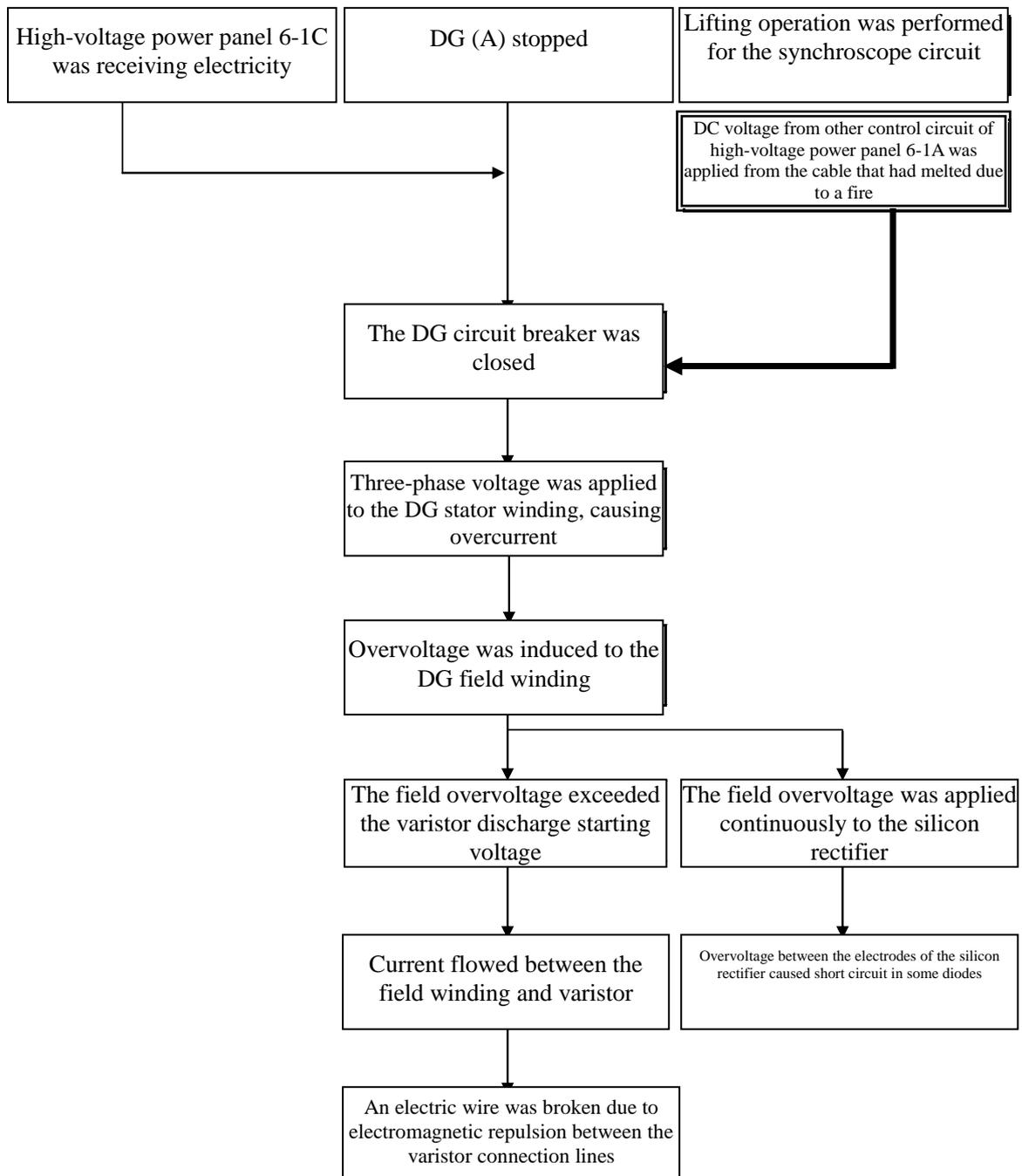
Fig. II-2-154 Varistor and rectifier mechanisms
