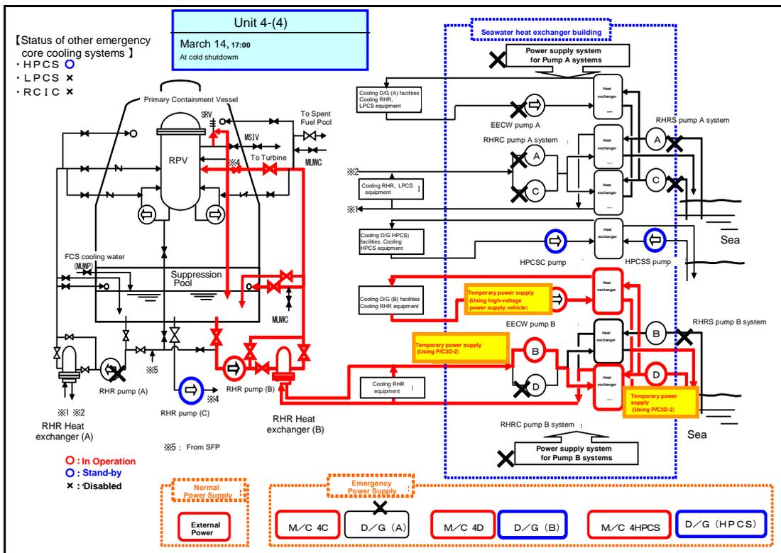
Figure II-2-123 Schematic Diagram of Station Status [2F-4] (Part 2)
