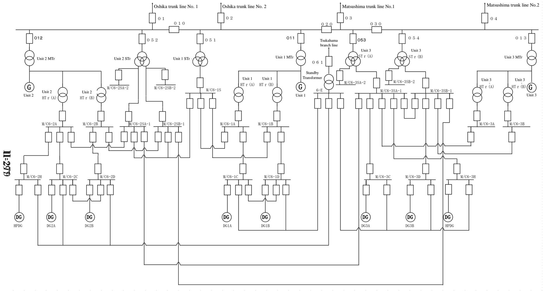
Figure II-2-130 Schematic Diagram of Distribution System of Onagawa NPS (Units 1 to 3)
