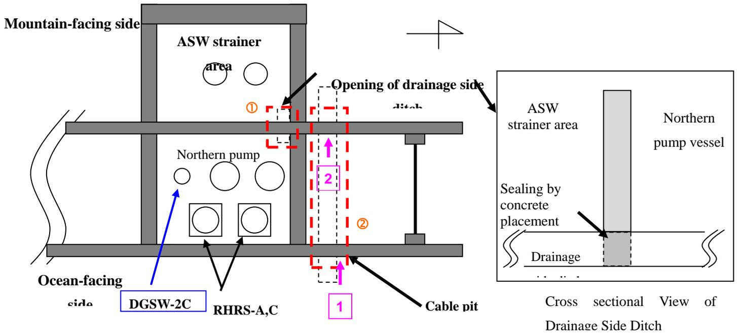
**Measure 1: Ensuring water tightness by concrete placement to the opening of drainage side ditch**
