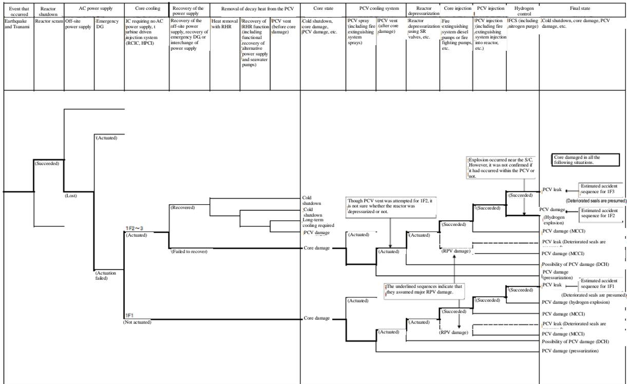
Fig.II-2-177 Functional Event Tree for Fukushima Dai-ichi NPS Units 1 to 3
