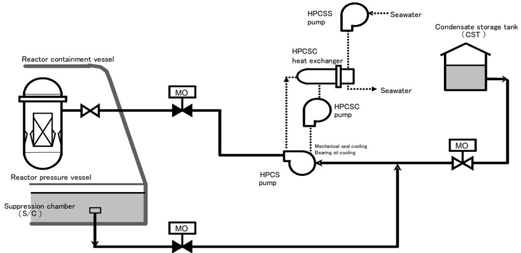
Figure II-2-87 System Diagram of High Pressure Core Spray System (Units 1 and 3)
