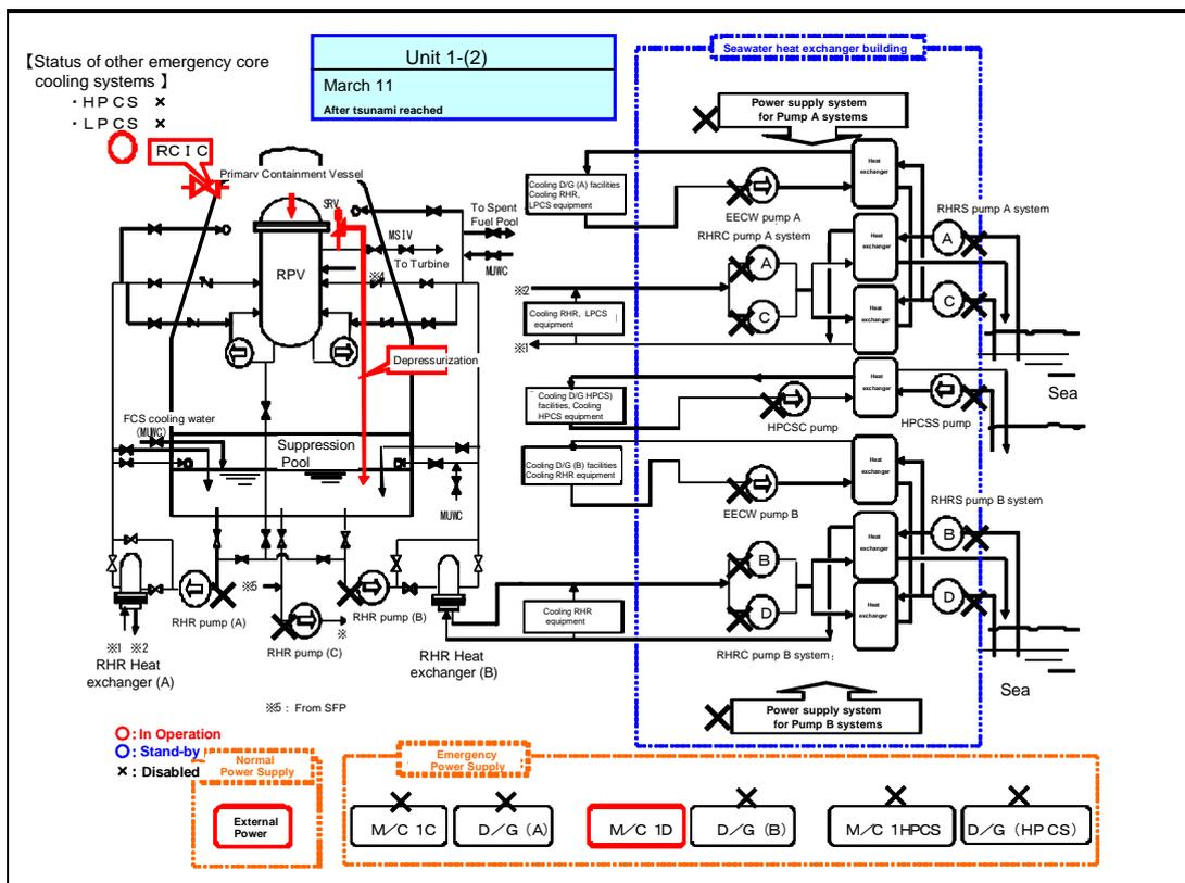
Figure II-2-107 Schematic Diagram of Station Status [2F-1] (Part 1)
