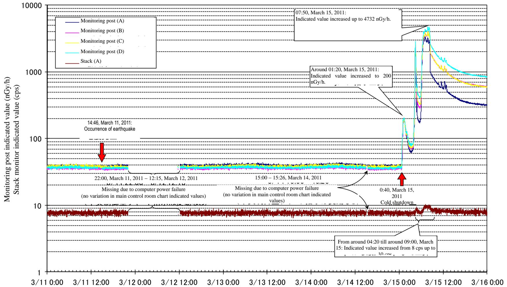
Figure II-2-165 Transition of Indicated Value of Monitoring Posts (from March 11 till March 15) (No. 1)
