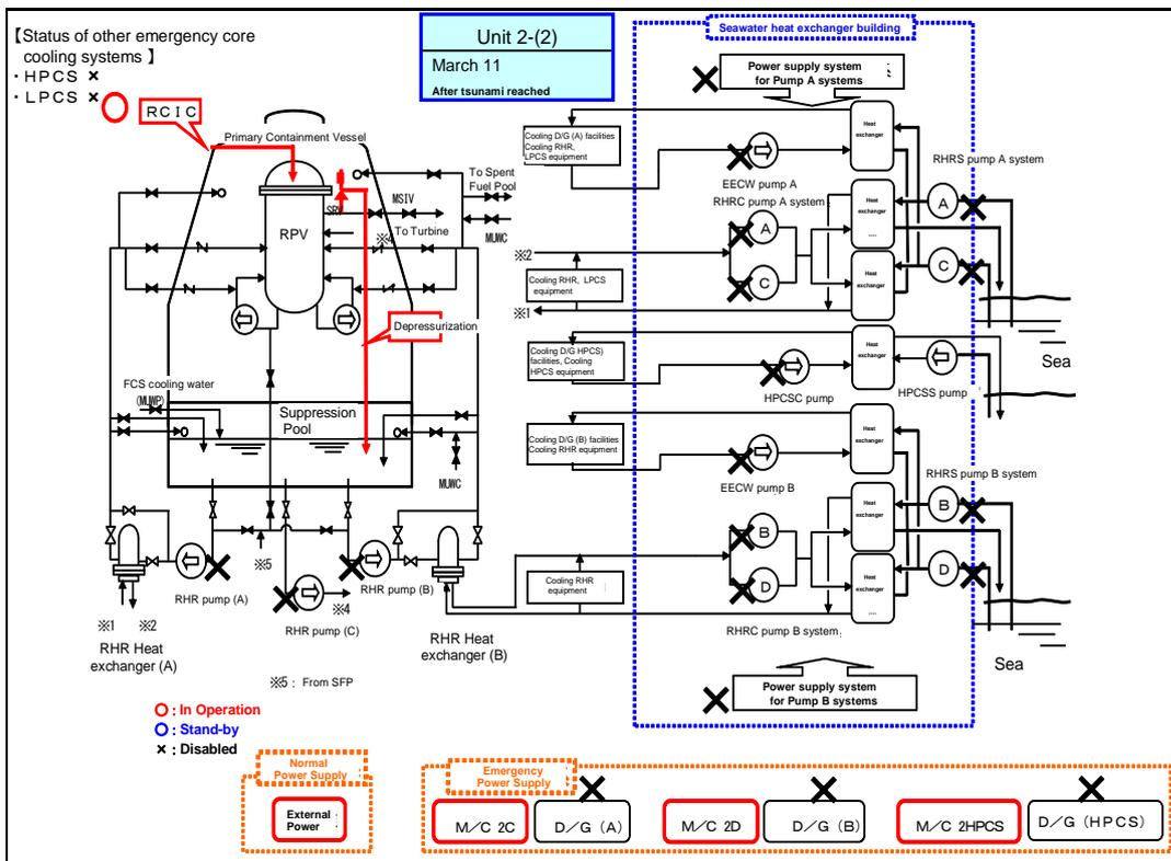
Figure II-2-112 Schematic Diagram of Station Status [2F-2] (Part 1)
