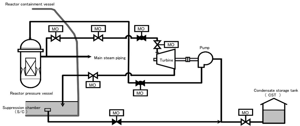
Figure II-2-91 System Diagram of Reactor Core Isolation Cooling System (All Units)
