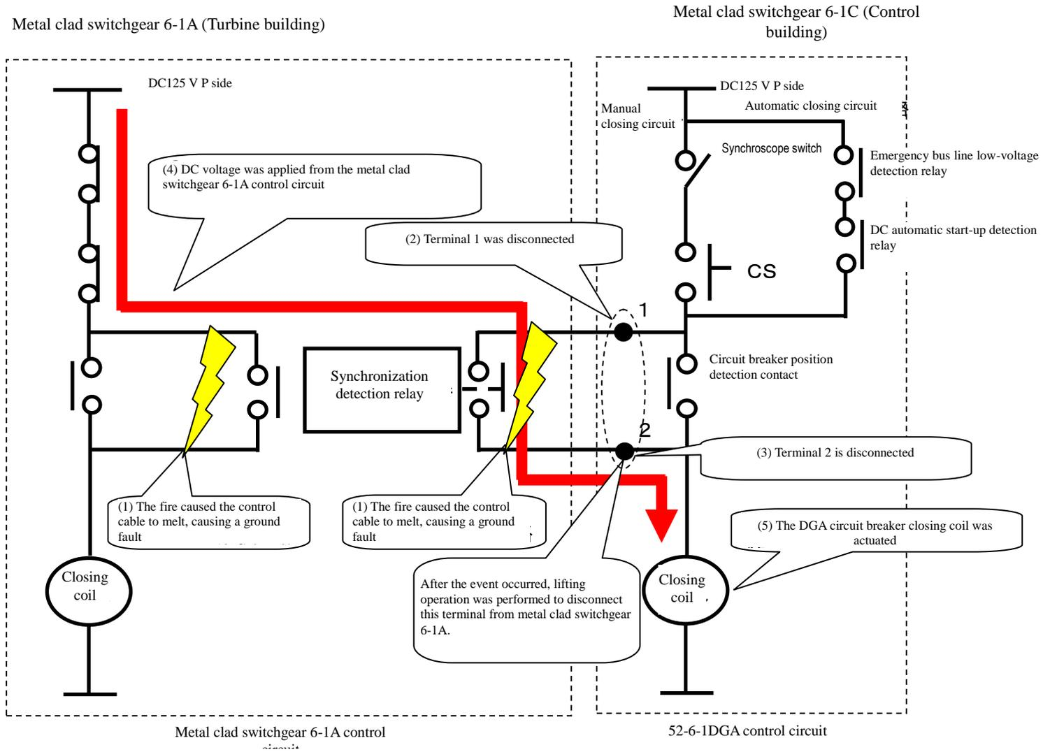
Fig. II-2-153 How the circuit breaker automatically closed
