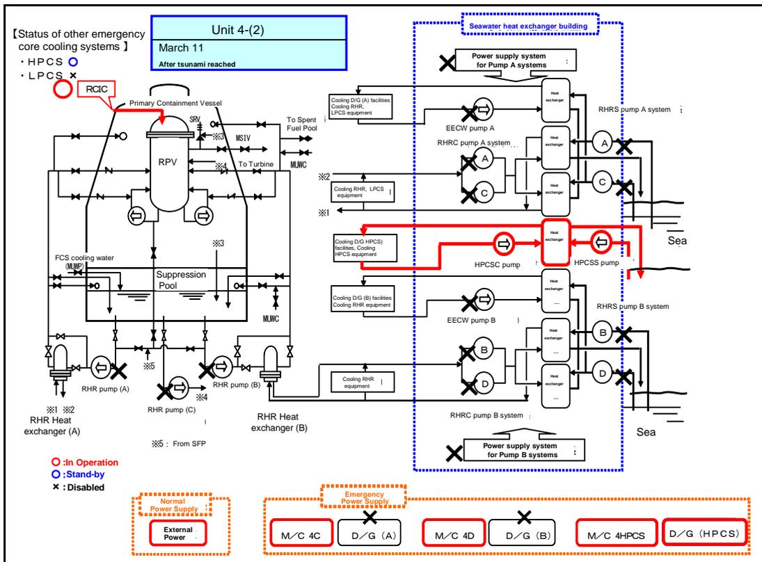
Figure II-2-122 Schematic Diagram of Station Status [2F-4] (Part 1)
