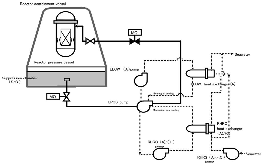
Figure II-2-90 System Diagram of Low Pressure Core Spray System (Units 2 and 4)
