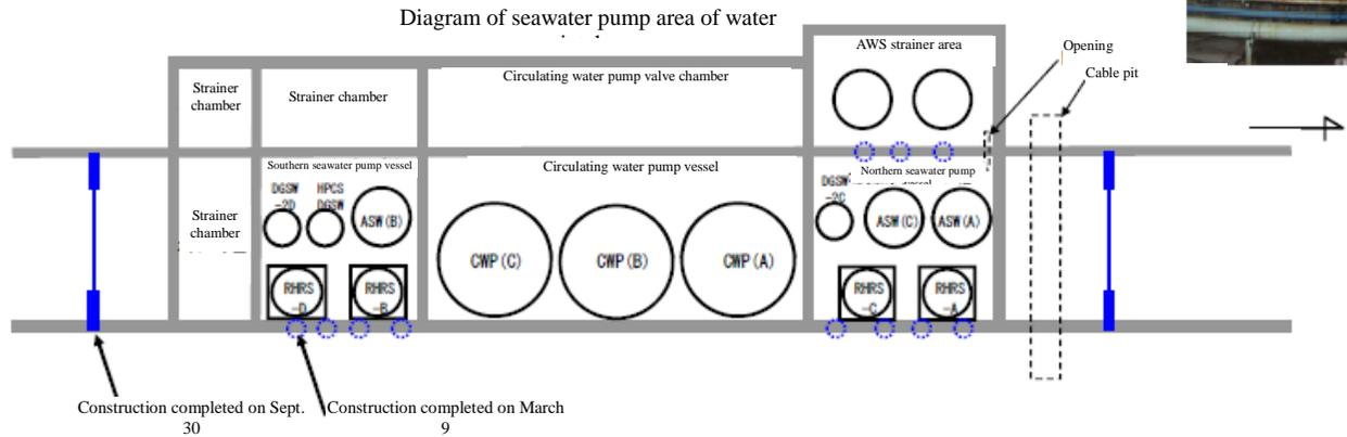
Fig. II-2-172 Status of Construction at Seawater Pump Area for Anti-tsunami Measures When Earthquake Occurred (March 11)
