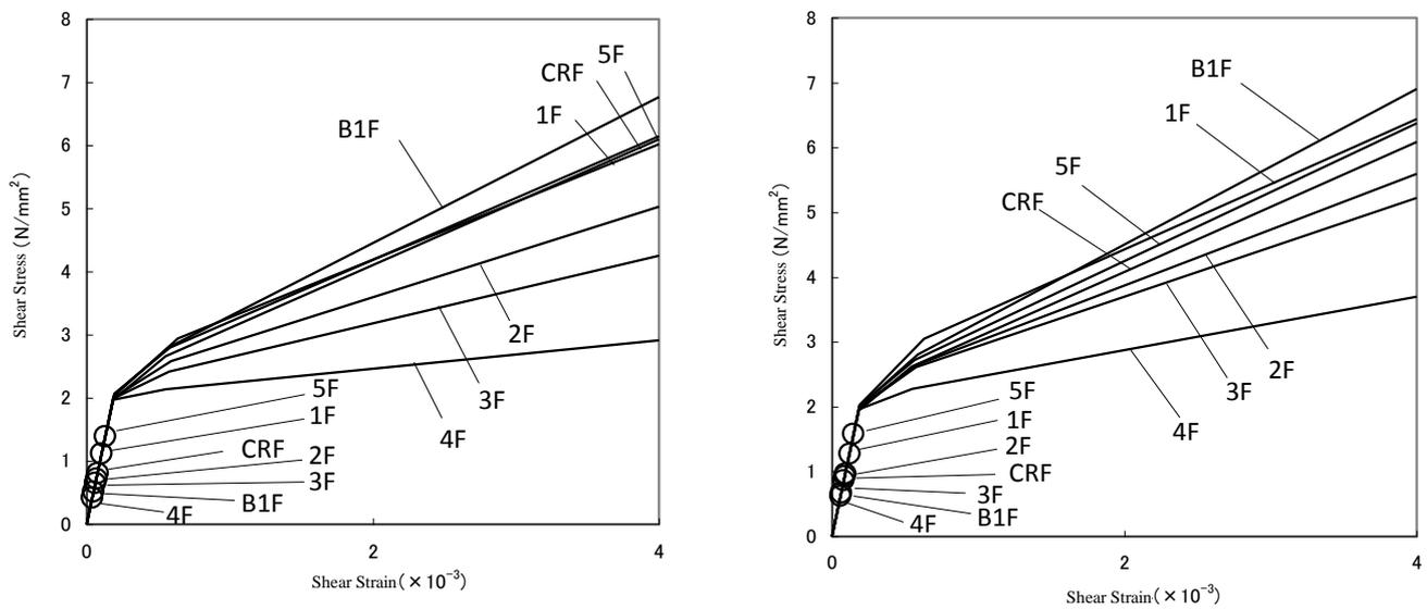
Figure II-2-11 Shear Strain on Seismic Wall (Left: NS Direction, Right: EW Direction)
