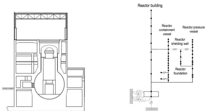
Figure II-2-14 Example of Model for Building-Large Equipment Interaction Response Analysis
