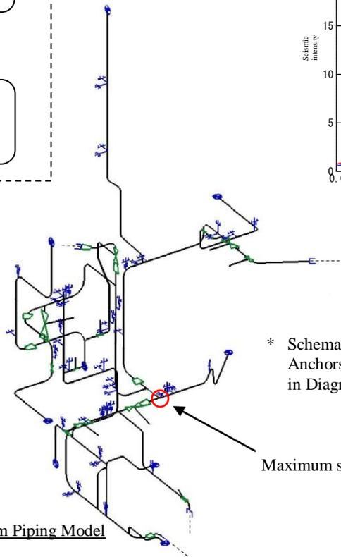
Residual Heat Removal System Piping Model
