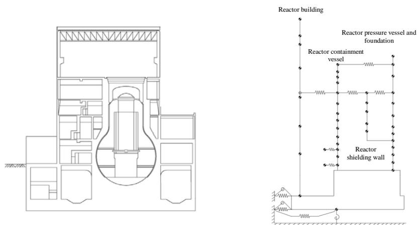
Figure II-2-18 Example of Model for Building-Large Equipment Interaction Response Analysis
