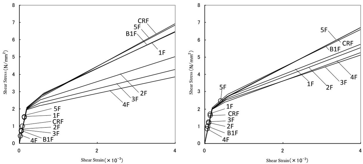
Figure II-2-9 Shear Strain on Seismic Wall (Left: NS Direction, Right: EW Direction)
