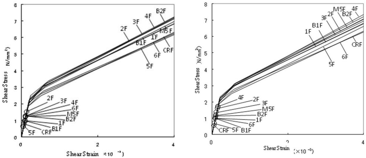
Figure II-2-13 Shear Strain on Seismic Wall (Left: NS Direction, Right: EW Direction)
