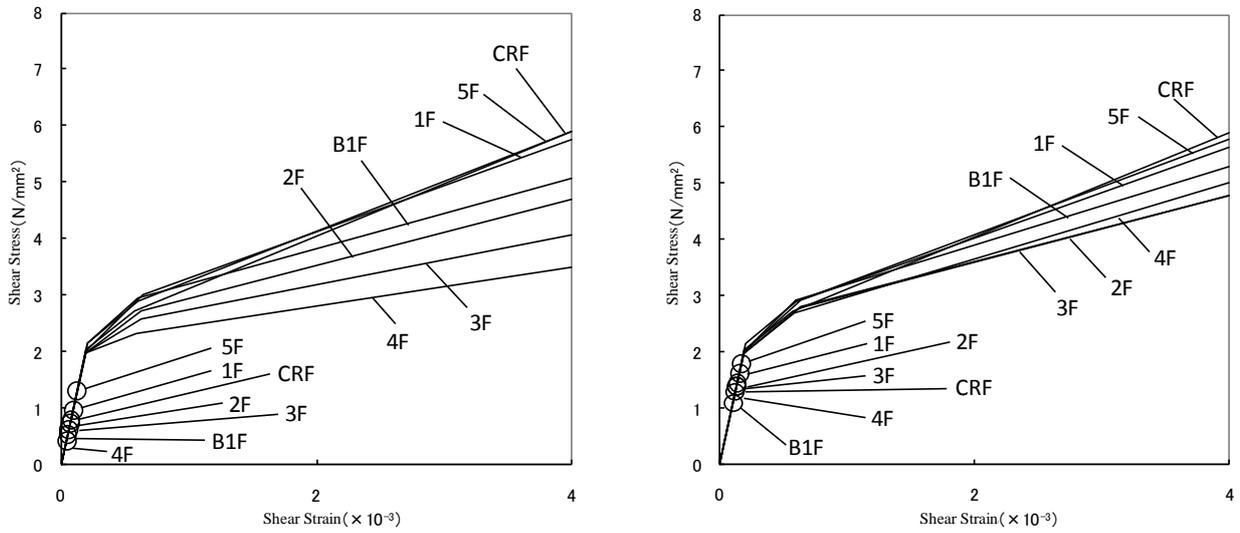
Figure II-2-10 Shear Strain on Seismic Wall (Left: NS Direction, Right: EW Direction)
