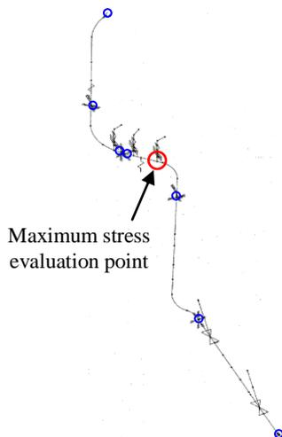
Main Steam System Piping Model (Partial View)
