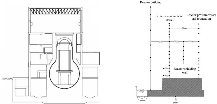
Figure II-2-16 Example of Model for Building-Large Equipment Interaction Response Analysis
