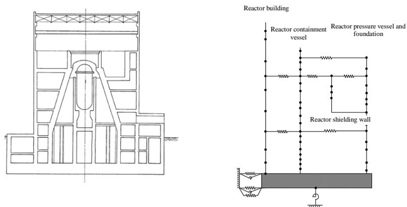
Figure II-2-19 Example of Model for Building-Large Equipment Interaction Response Analysis
