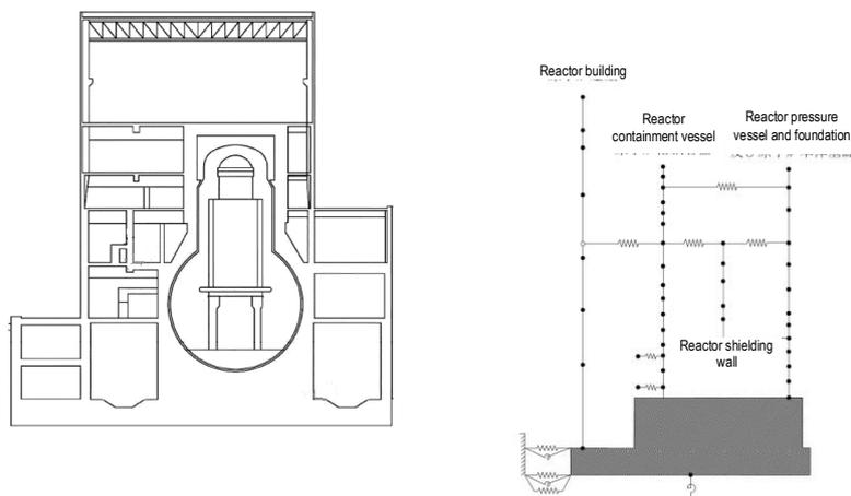
Figure II-2-15 Example of Model for Building-Large Equipment Interaction Response Analysis
