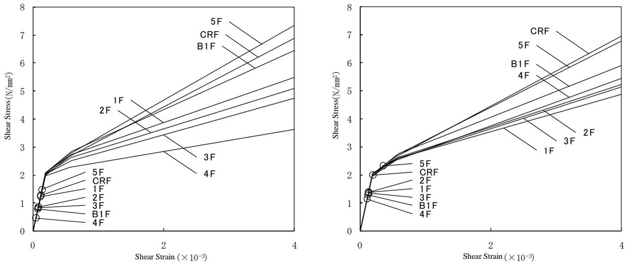
Figure II-2-12 Shear Strain on Seismic Wall (Left: NS Direction, Right: EW Direction)
