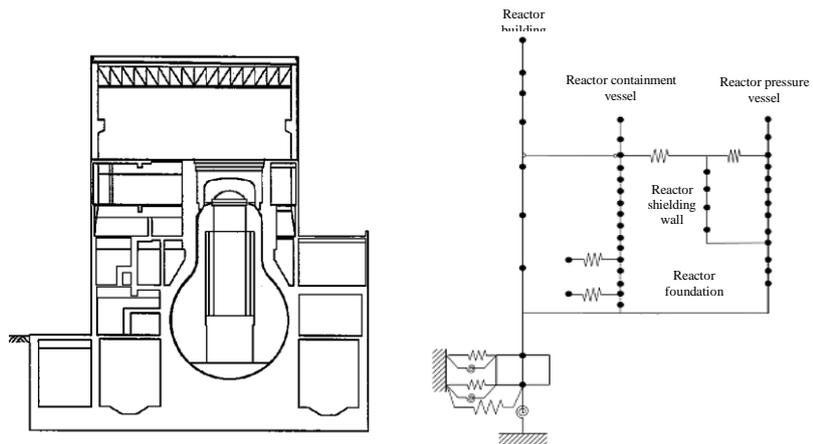
Figure II-2-17 Example of Model for Building-Large Equipment Interaction Response Analysis
