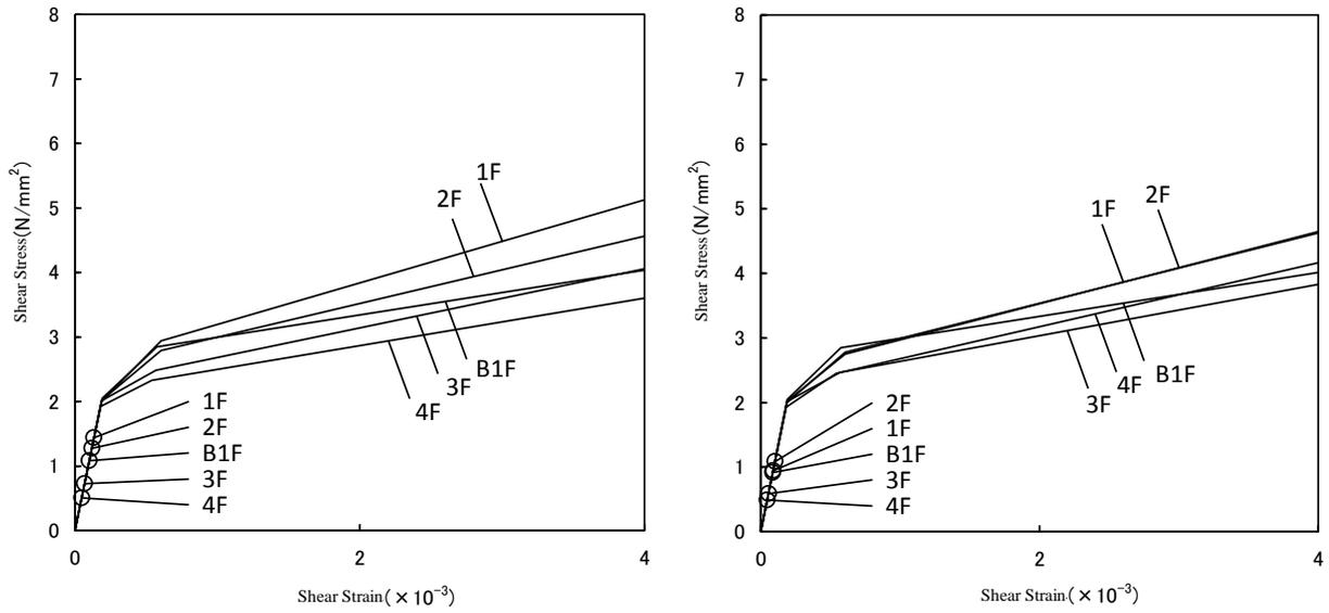
Figure II-2-8 Shear Strain on Seismic Wall (Left: NS Direction, Right: EW Direction)
