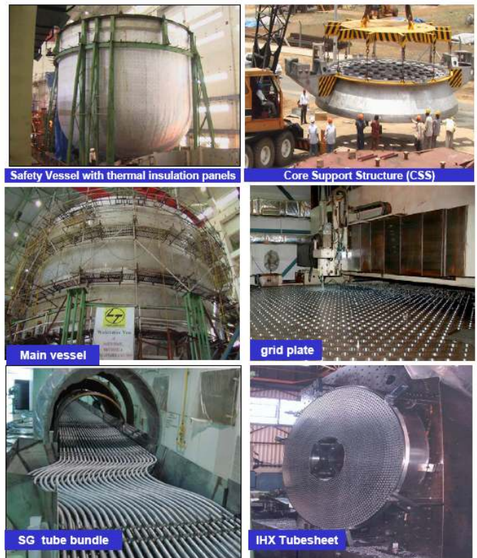
Progress made with component manufacturing for India's Prototype Fast Breeder Reactor (PFBR) under construction at Kalpakkam [courtesy of Indira Gandhi Center for Atomic Research (IGCAR) and Bharatiya Nabhikiya Vidyut Nigam Ltd (BHAVINI)]
