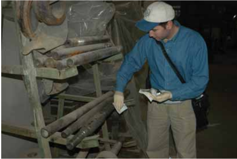
FIG. 4. Taking environmental samples at a nuclear facility.
