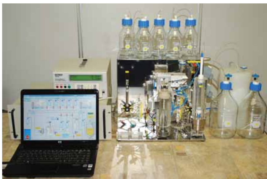
FIG. 1. 'Kamadhenu', a fully automated strontium-90/yttrium-90 electrochemical generator designed and built by Isotope Technology Dresden using technology developed through an Agency CRP. (Photograph courtesy of J. Comor.)
