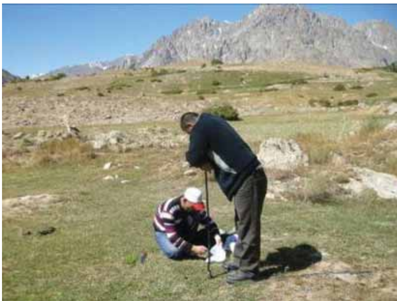
FIG. 2. Taking soil samples from the High Pamir Mountains of Tajikistan to assess spatial FRN distribution and hence soil erosion deposition. (Photograph courtesy of Lomonosov Moscow State University, Russian Federation.)
