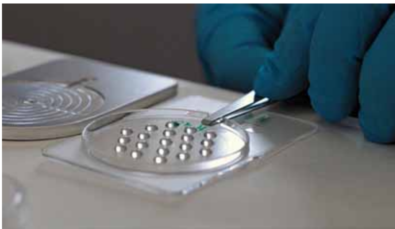
FIG. 4. Preparation of simulated air filter reference material for the ALMERA proficiency test.
