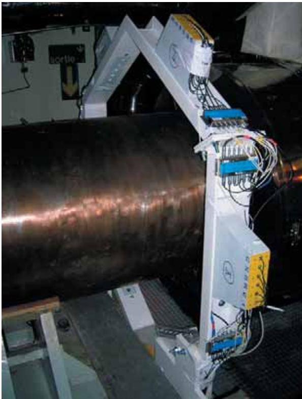
FIG. 2. A single photon emission computed tomography system in a French nuclear power plant. The system, installed around the primary circuit of a PWR, improves the estimation of nuclear thermal power in correlation with nitrogen-16 activity produced from oxygen-16 in water.
