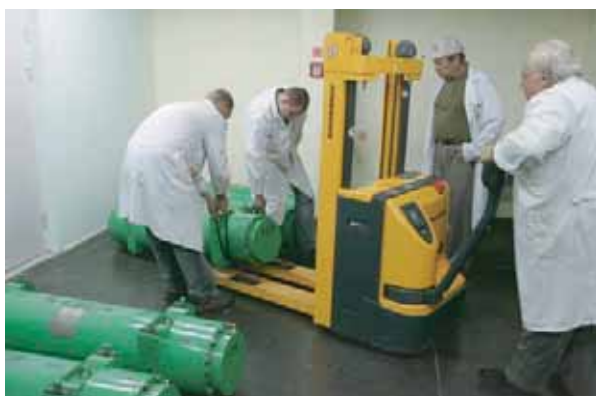
FIG. 1. Handling a transport cask with fresh HEU prior to shipment back to the Russian Federation under the RRRFR programme.
