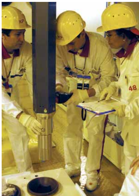
FIG. 1. Nuclear safeguards inspectors verifying the active length of a fresh fuel assembly using a gamma ray system at the Mochovce nuclear power plant, in Slovakia, during a training exercise.
