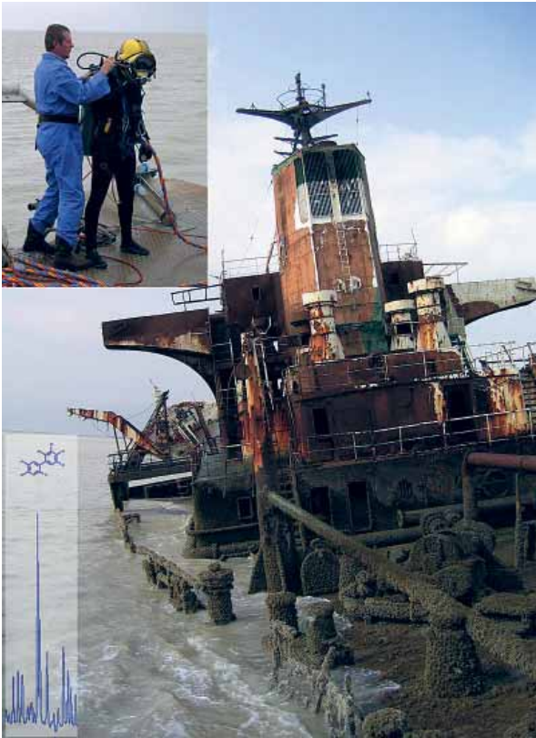
FIG. 2. Pollution sampling (top inset) and chromatographic analysis (lower inset) of sediments collected at one of the 35 shipwrecks located in and around Iraqi waterways.
