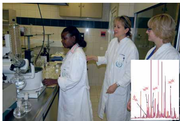
FIG. 1. Research and training at IAEA-MEL on pesticide extraction from marine biota. Shown in the inset is the gas chromatographic separation and detection of individual pesticides.
