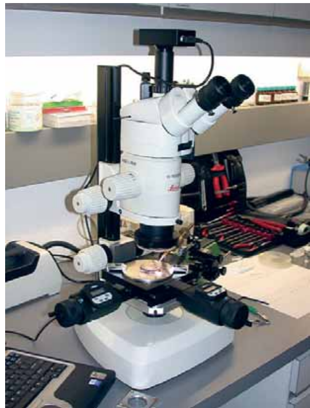
FIG. 3. The microparticle manipulation system assembled at the Agency's Laboratories at Seibersdorf.
