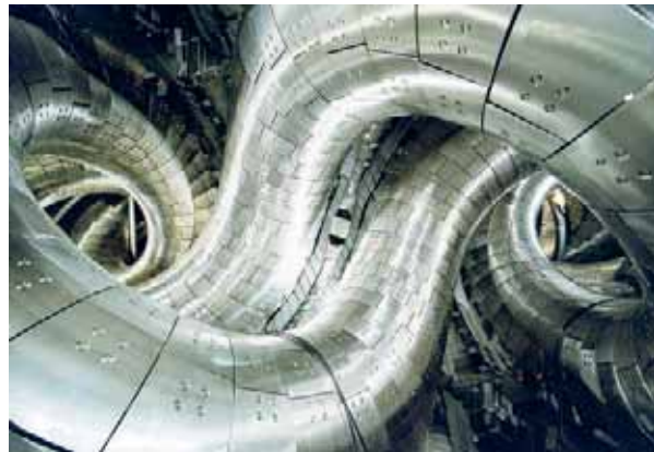
FIG. 2. Inside view of the Japanese stellarator LHD vacuum chamber — a toroidal nuclear fusion confinement concept — showing the covered helical winding of the coil system. The fusion plasma is confined by the coils inside the vacuum chamber.
