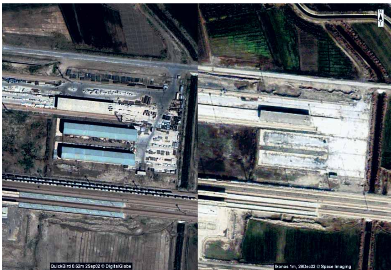
FIG. 1. An example of satellite imagery used for change detection analysis, which involves comparing a site on two different dates in order to update the Agency's knowledge with regard to the site infrastructure and contents. The picture on the left is from the QuickBird satellite at an altitude of 450 km, while the image on the right is from the Ikonos satellite at an altitude of about 680 km (copyright: QuickBird DigitalGlobe; and Ikonos Space Imaging).
