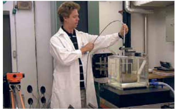
FIG. 3. Accuracy of radiation dose measurements is vital in radiotherapy. Here, a physicist at the Agency's Laboratories at Seibersdorf calibrates a dosimeter to be used in a Member State.
