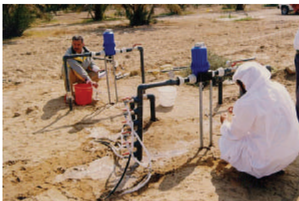
FIG. 1. On the basis of results from an Agency technical co-operation project, drip irrigation systems are beginning to replace surface irrigation schemes in arid areas. Shown here is a drip irrigation system in the Syrian Arab Republic.
