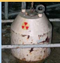
Sealed source transportation container in poor condition / V. Friedrich (IAEA)
