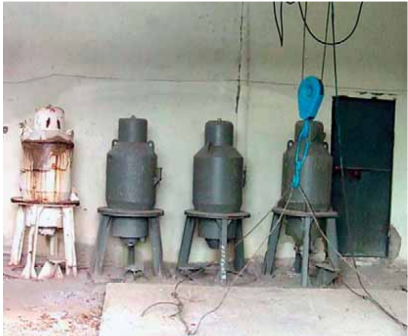
Sources used in mobile caesium irradiators in the former Soviet Union containing 130 TBq (~3500 Curies) of caesium-137. (Soviet Union)/IAEA
