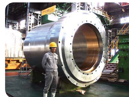
Industrial machine: Main cylinder for press, JSW Steel Forgings and Castings.
