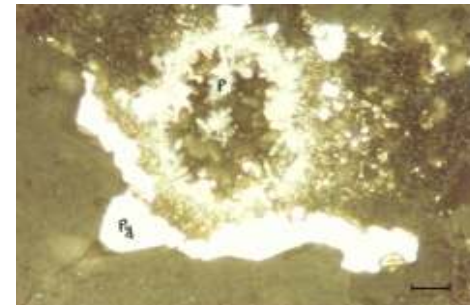
Ovoid grain showing intimate association of pitchblende (P) and pyrite (Py) in phosphatic siliceous calcitic dolostone
