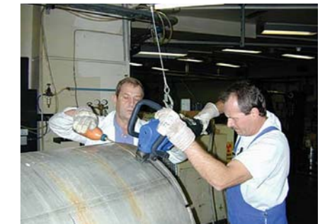
Use of nibblers in segmenting nuclear components
