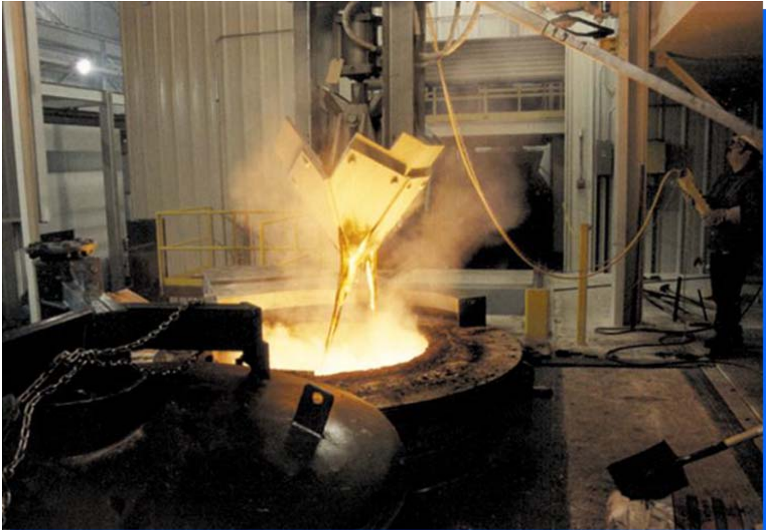
EnergySolutions' 20-ton, 7200 kW electric-induction furnace is the largest unit for melting and recycling radioactively contaminated metal in the U.S.
