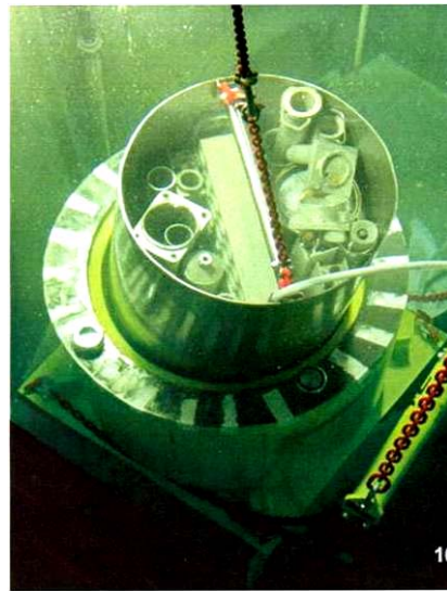
Under water loading of Mosaik Container 1811 Activity contents 370 GBq Co-60
